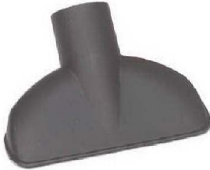
Figure 5: Picture of the nozzle used for the second flow seeding attempt.
