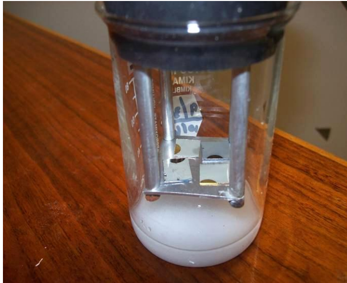
Figure 44: Sputtered Sn film coupons exposed to saturated aqueous salt solution.
