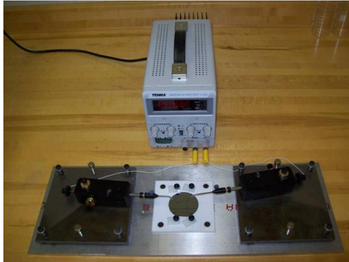
Figure 68: Probe station setup for steady current exposure through Sn pattern.
