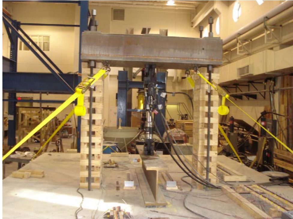
Figure 5-5: Fully Assembled Load Testing Frame Side View
