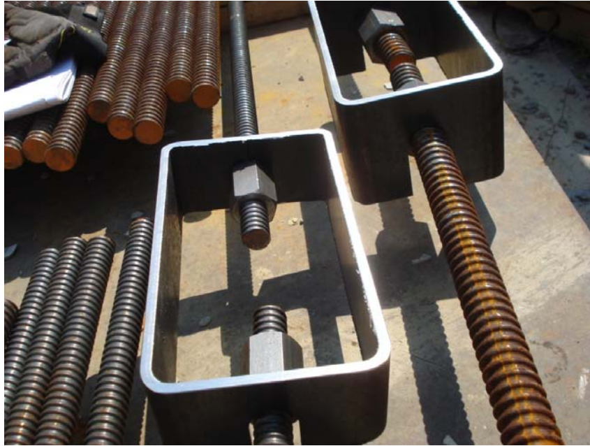
Figure 4-2: Test Fit of HSS Coupler: Staged Construction (left) and Transverse (right) End Elevation
