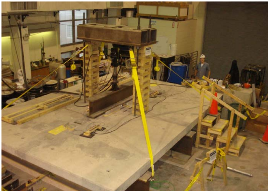
Figure 5-4: Fully Assembled Load Testing Frame from Above
