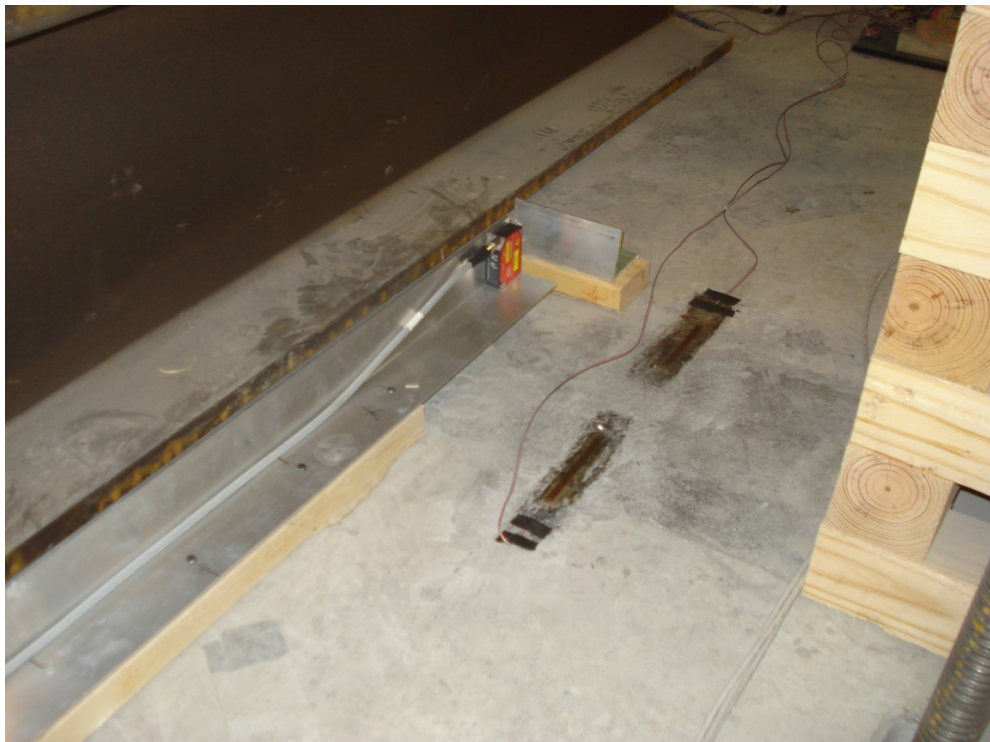
Figure 5-11: Typical Concrete Strain Gage and Laser Displacement Gage
