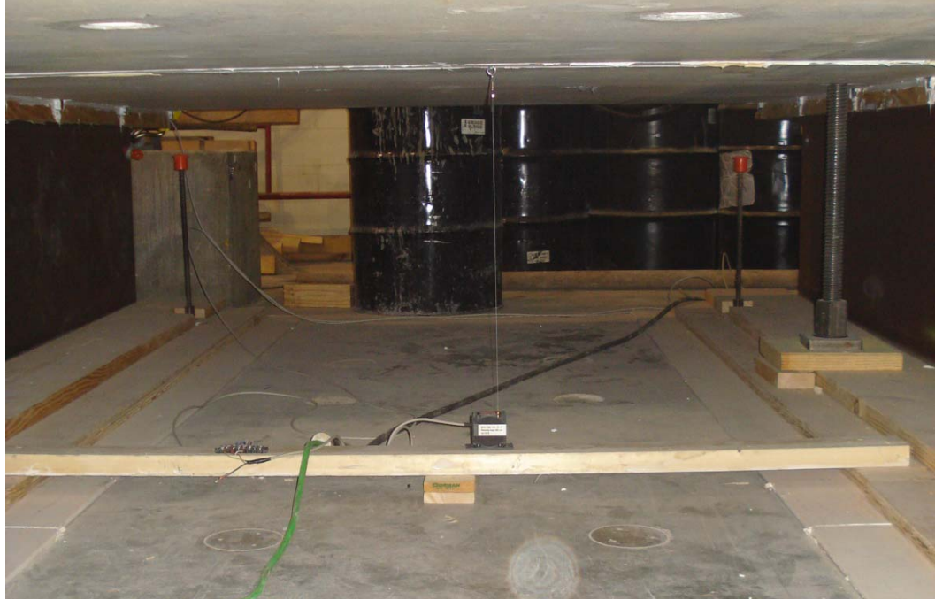
Figure 5-10: Typical Under-Slab Drawstring Displacement Gage Application
