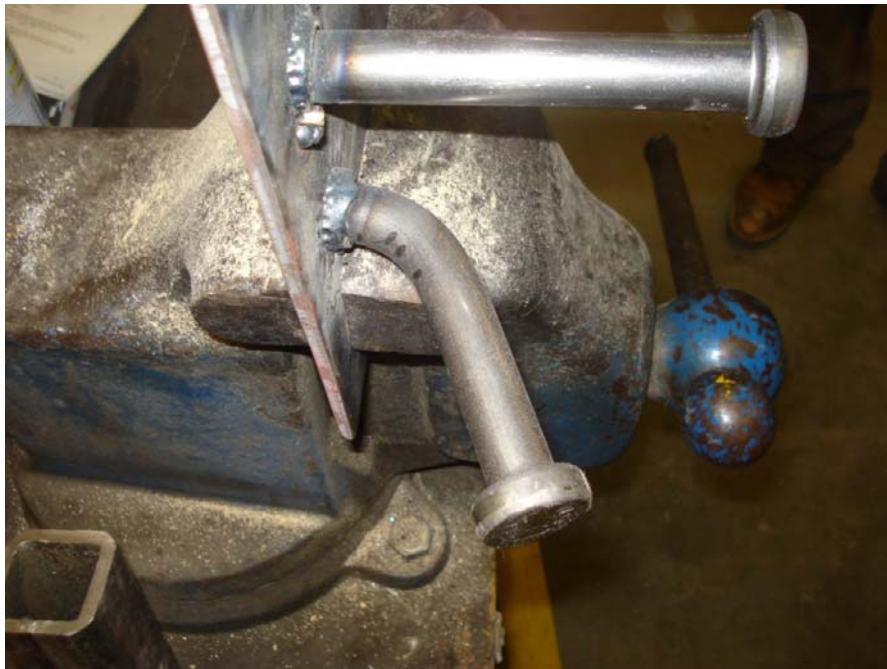
Figure 4-7: Shear Stud Quality Control Bend Test
