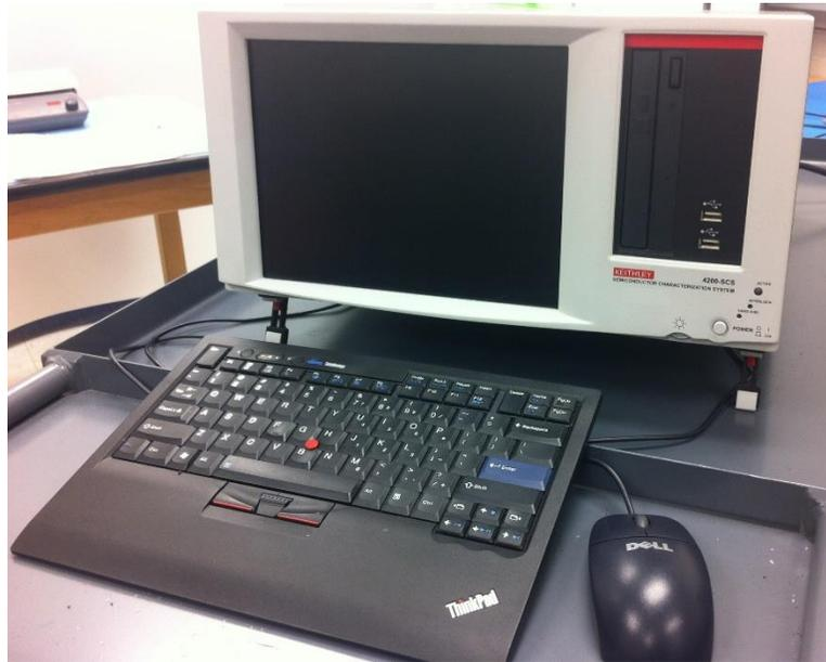
Figure A.7: Keithley 4200 (Semiconductor Characterization Systems) parameter analyzer.
