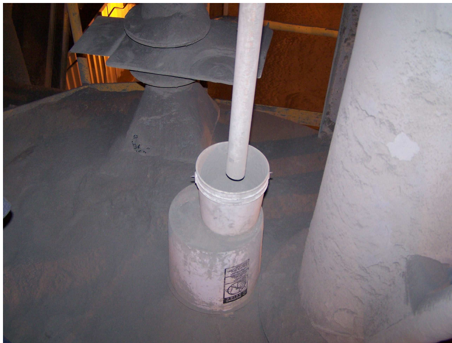
Figure 3.11: Automated Plunger Collecting Cement Samples
