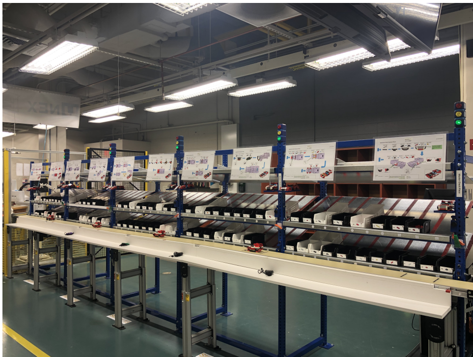
Figure 4.4: Cell-3 of the Lean education lab. The production stations from 11 to 15 are designed & assembled in this cell.
