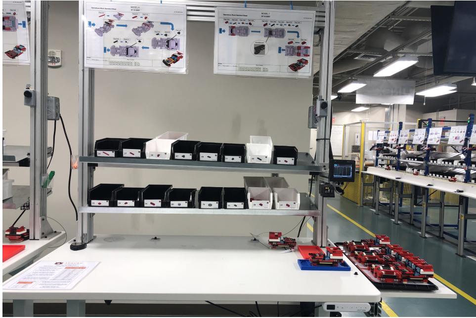
Figure 4.5: The production station 10 of the Lean education lab. The interaction between Lean (mistake-proof) and I-4.0 (vision technology) was performed at this station.
