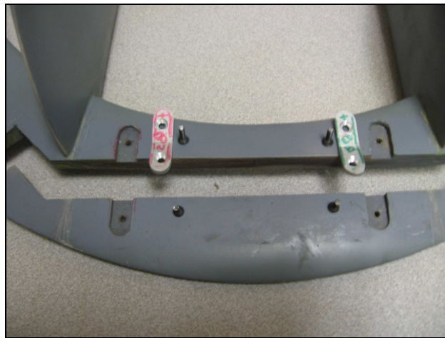
Figure 3.3 Elevator hardware construction
