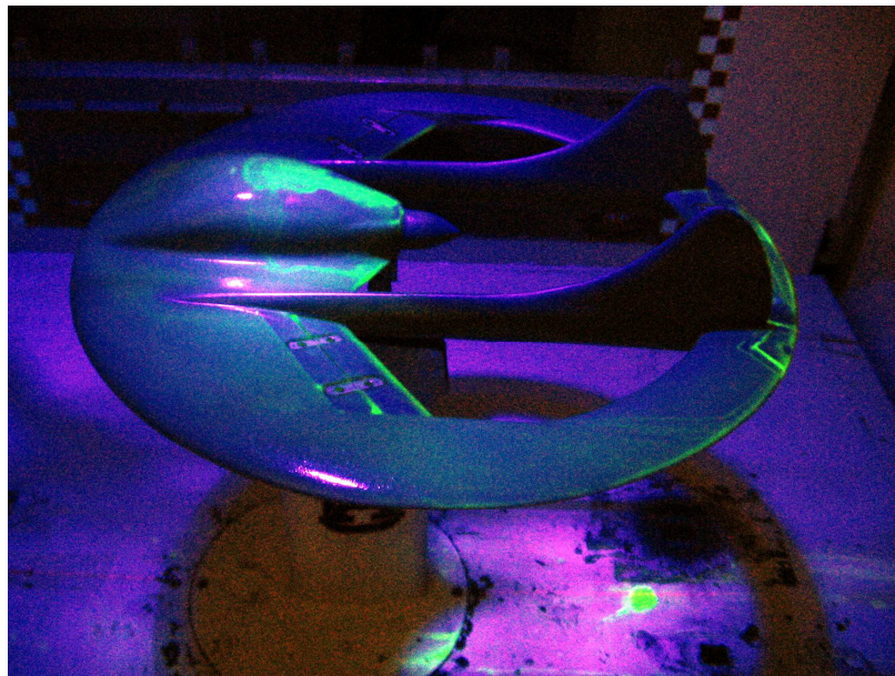
Figure 5.27 Geobat flow visualization at \alpha = 0 deg
