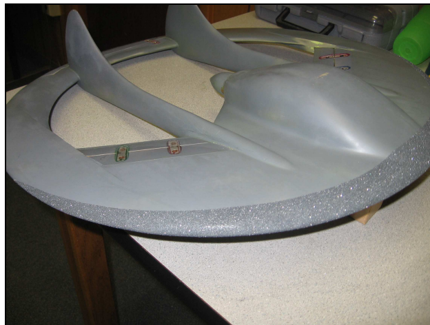
Figure 3.6 Final transition strip
