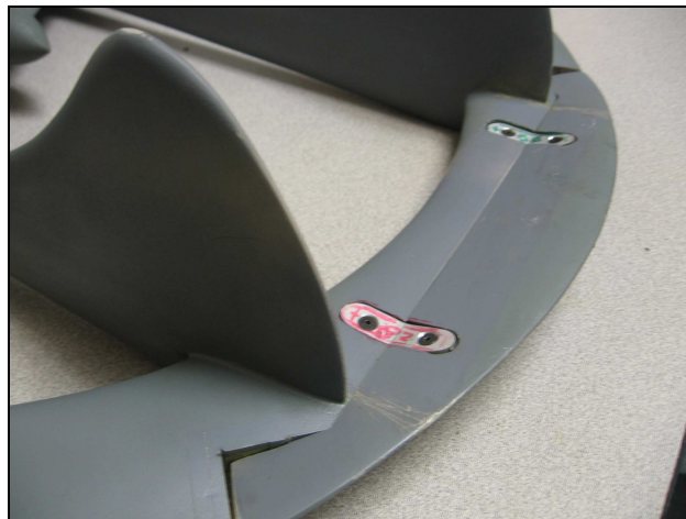
Figure 3.4 Attached elevator with hardware
