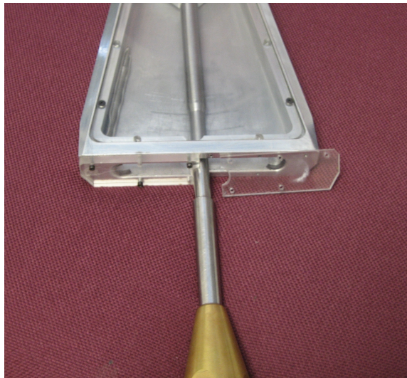
Figure 2.4: Close up of the acrylic plates used to lock the yaw motion.
