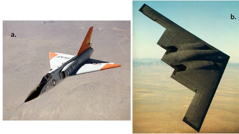
Figure 1.1: Different delta wing planforms: a.) Slender[1] b.) Non-slender[2].
