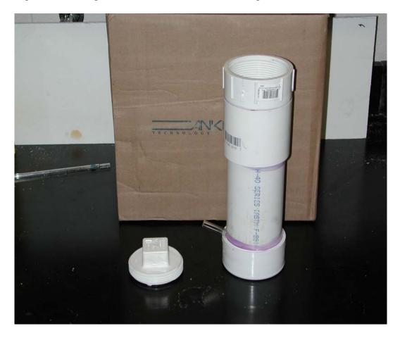
Figure 2.1: Fumigation Chamber used in 2005-2006 greenhouse studies.
