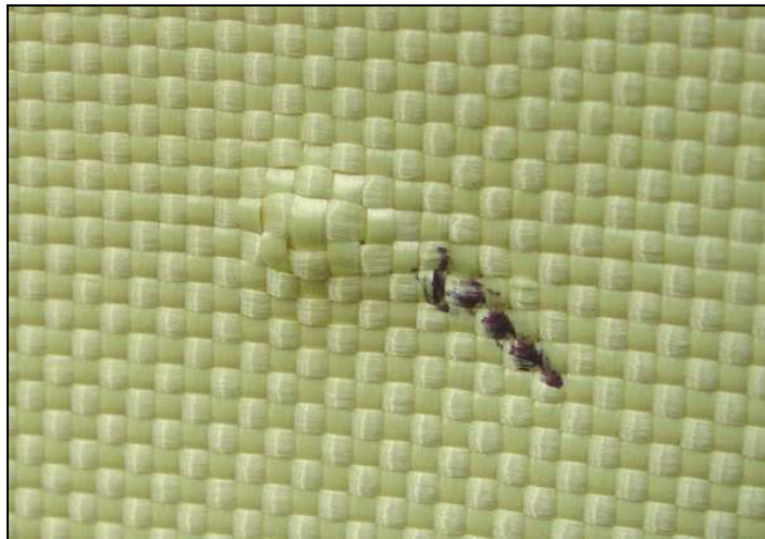
Figure 47. Backface Deformation of the Target through Reflection (Target: 2BG-Laminated, Bullet: 0.22 Short)
