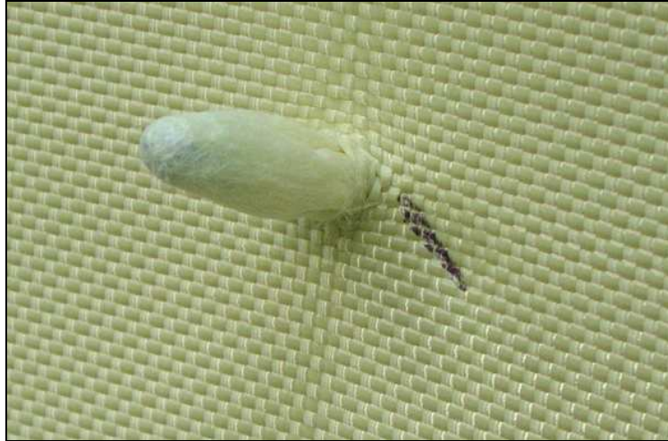
Figure 44. Transit of Nonwoven Layer through the Target III (target: 2BG+1NW, bullet: 0.22 Short)
