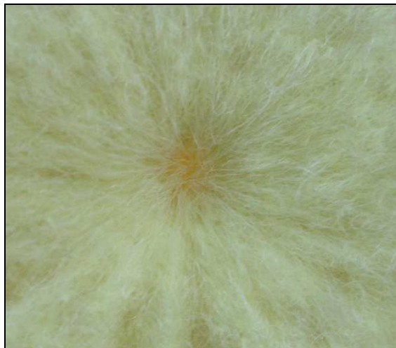
Figure 43. Transit of Nonwoven Layer through the Target II (target: 1BG+1NW, bullet: 0.22 Short)
