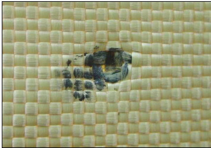
Figure 46. Bullet Mark on the Front Face of the Target after Reflection (target: 2BG-Laminated, bullet: 0.22 Short)
