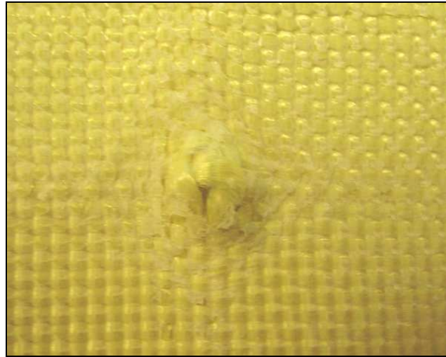
Figure 48. Delamination between the BG Fabrics in the Impact Zone
