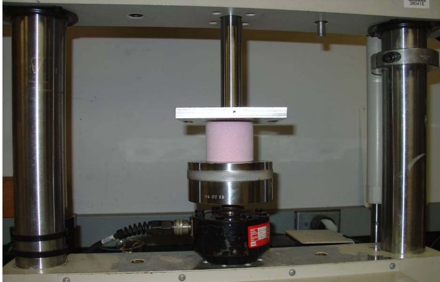
Fig. 3.3. Testing configuration for foam
