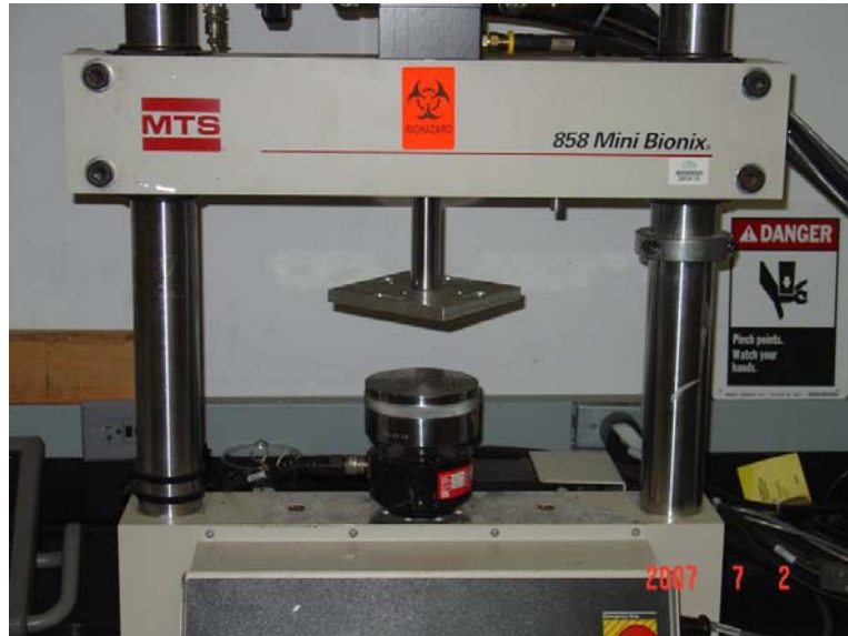
Fig. 3.1. Test equipment for foam
