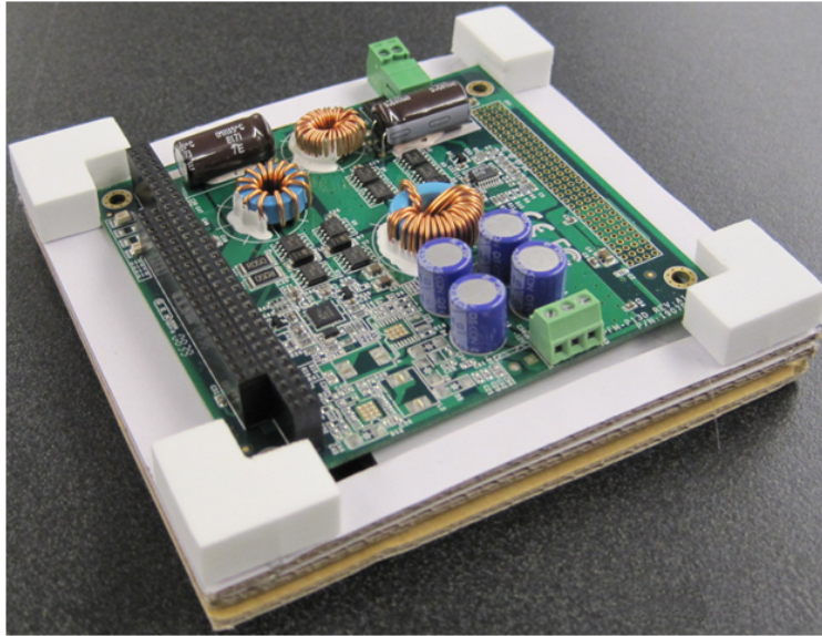
Figure 13.3: This figure shows a view of the PC104 Power Supply module from the top.
