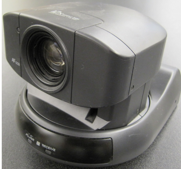
Figure 13.15: This figure shows the Sony EVI-D30 Pan-Tilt-Zoom camera controlled by the camera controller External Agent.
