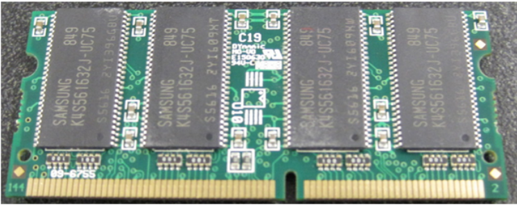
Figure 13.7: This figure shows the 256MB, 144 pin Synchronous Dynamic RAM high-density memory module which is the RAM of the PC104 sensor node.
