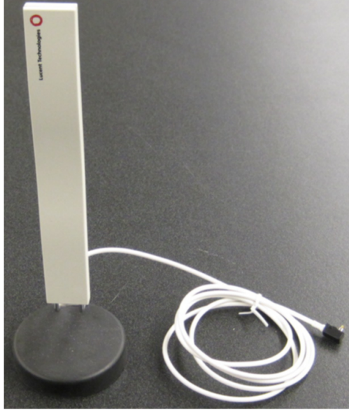
Figure 13.5: This figure shows a view of the Lucent omnidirectional external antenna used to boost the signal range of the wireless sensor nodes.
