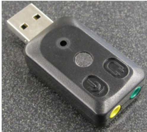
Figure 13.8: This figure shows the USB microphone which acts as an acoustic sensor for the PC104 sensor node.
