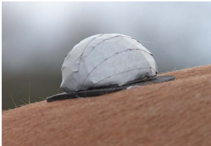
Figure 3.3: Three dimensional markers comprised of one-half of a styrofoam ball covered with Scotchlite 8850 retroreflective tape (Motion Lab Systems, Inc., Baton Rouge, LA) and mounted on black foam were used along the vertebral column at the withers, lumbar-sacral junction, and point of the croup.
