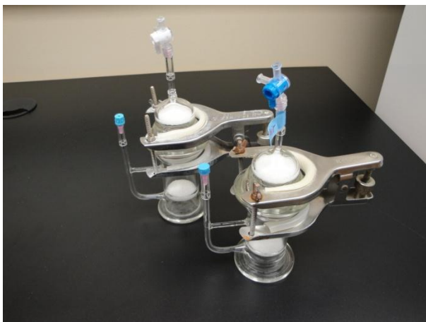
Figure 15. Odorant applicators for DMNB. The applicator allows delivering sublimation vapors from a solid DMNB (Courtesy of P. Waggoner)
