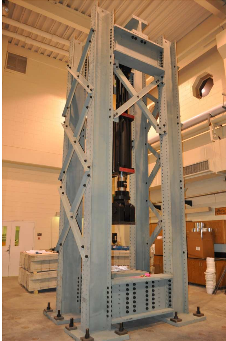
Figure 3-12 Load Testing Frame
