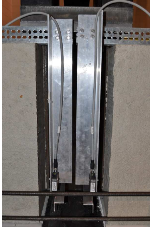
Figure 3-14b Photo of Instrumentation for Relative Slip Measurement
