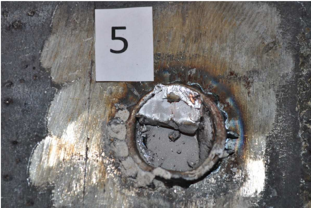
Figure 4-29 Failure Surface for S-0.875-22-A (5)
