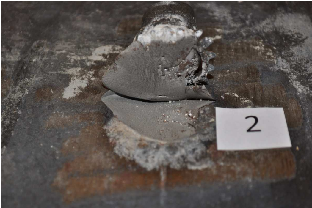
Figure 4-19 Failure Surface for S-0.875-18-A (2)
