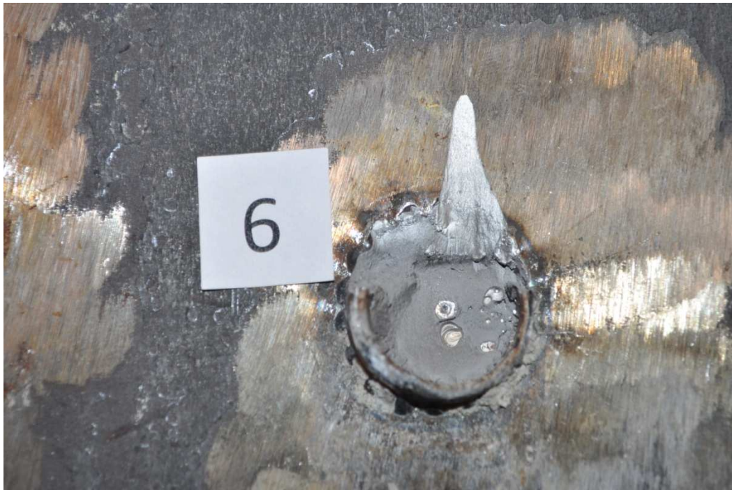
Figure 4-12 Failure Surface for S-0.875-22-B (6)
