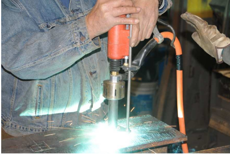
Figure 3-7 Drawn-Arc Welding Process Used for Stud Welding
