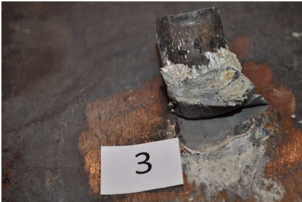
Figure 4-20 Failure Surface for S-0.875-18-C (3)
