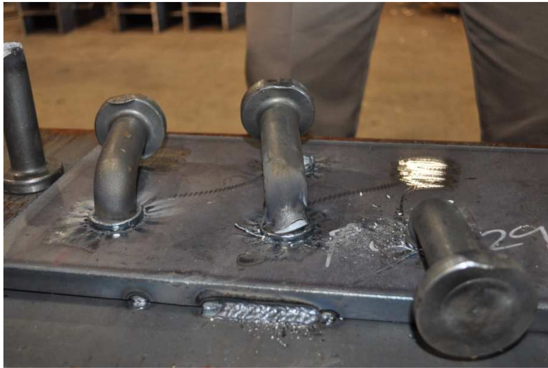
Figure 3-8 Bend Test Performed on 1¼"-Diameter Studs
