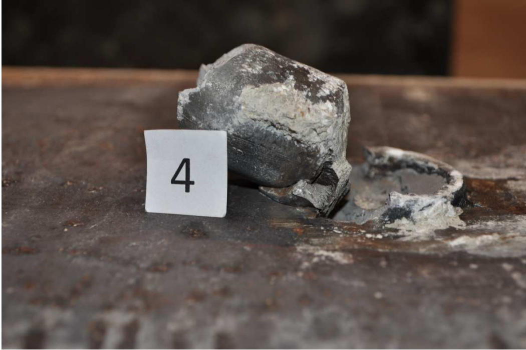
Figure 4-13 Failure Surface for S-1.25-22-B (4)
