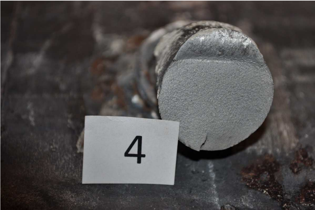
Figure 4-22 Failure Surface for S-1.25-18-B (4)
