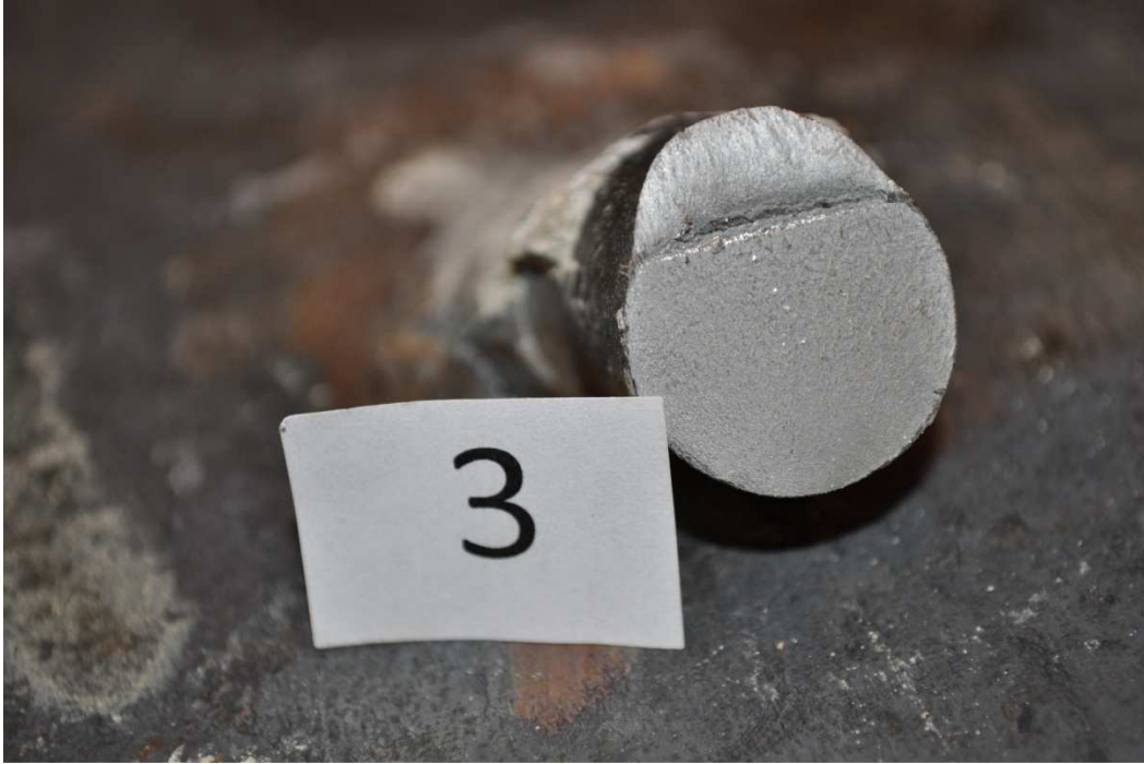
Figure 4-21 Failure Surface for S-0.875-18-C (3)
