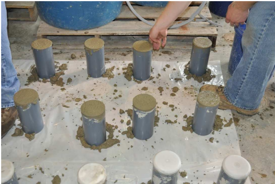
Figure 3-9 Making 4×8 Concrete Cylinders for Compression Tests
