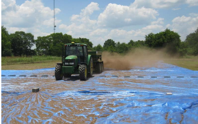
Figure 3.2. Tractor, litter spreader, and collection pan matrix used during pan testing.
