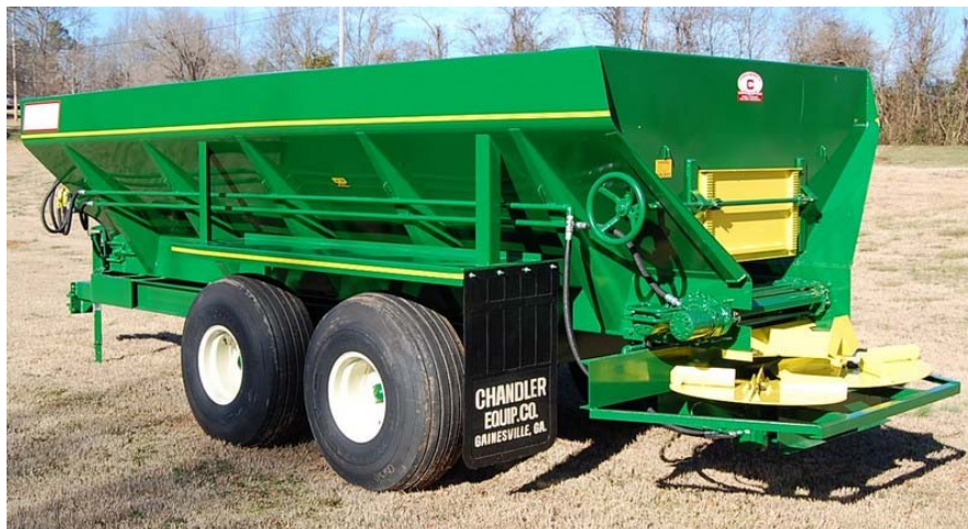
Figure 2.1. Typical spinner-disc spreader used for litter spreading.
