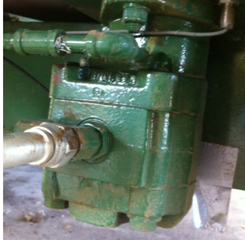
Figure D.4. Parker/Commercial Intertech hydraulic spinner motor.
