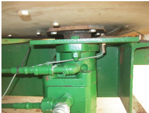
Figure E.3. Proximity sensor to monitor spinner-disc speed.
