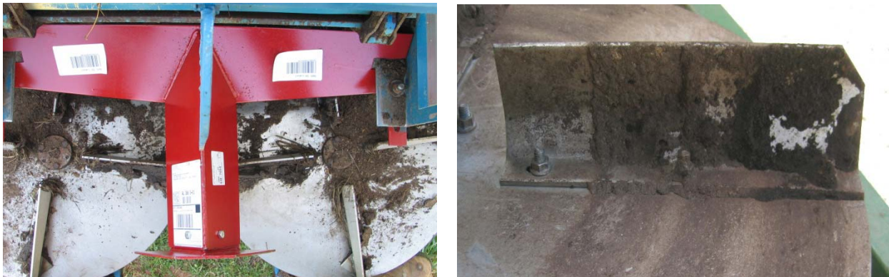
Figure 6.2. Illustration of litter buildup on spinner-discs and vanes.
