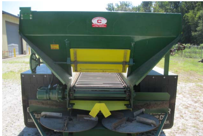
Figure D.3. Litter spreader rear gate, conveyor chain, flow divider and spinners.
