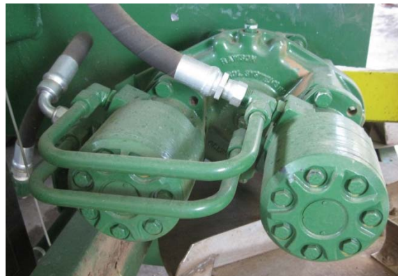
Figure D.5. Parker/Ross hydraulic conveyor motors.
