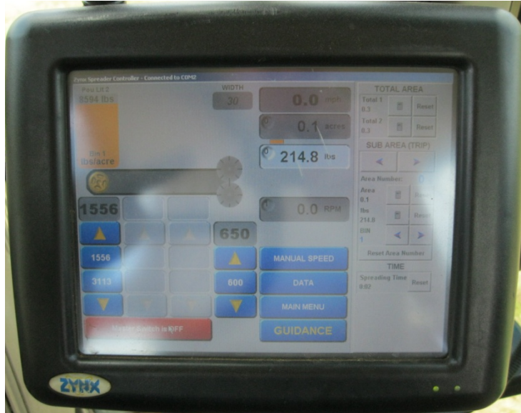
Figure E.1. Snapshot X20 console showing the main screen of the Spreader Control Software.
