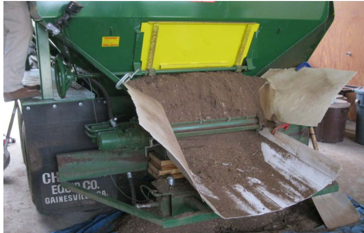
Figure 3.1. Spreader setup used during conveyance testing illustrating fabricated chute for funneling litter into the plastic, collecting container.
