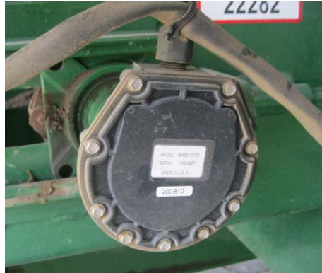
Figure E.4. Encoder to monitor conveyor speed.
