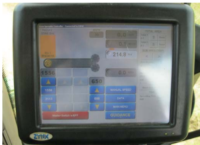
Figure 2.3. Example of a display-rate controller (Topcon Precision Ag X20) commonly used for spinner-disc spreaders.
