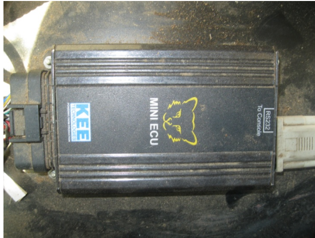
Figure E.2. Electronic Control Unit (ECU) used with a litter spreader.
