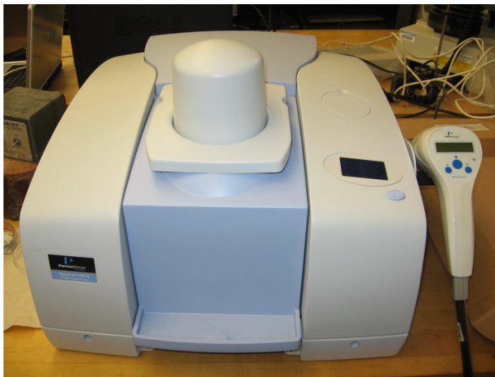
Figure 5.1. FT-NIR spectrometer used for collecting spectral data of broiler litter.
