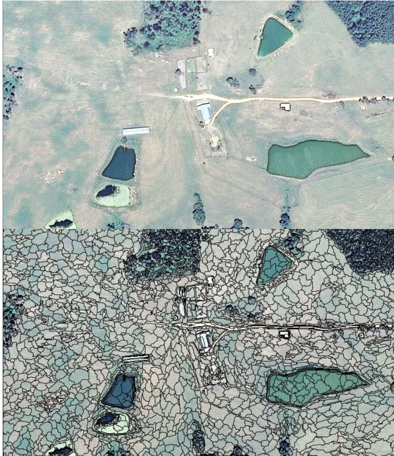
Figure3.1 This image shows the Multi-Resolutional Segmentation on a section of NAIP Imagery
