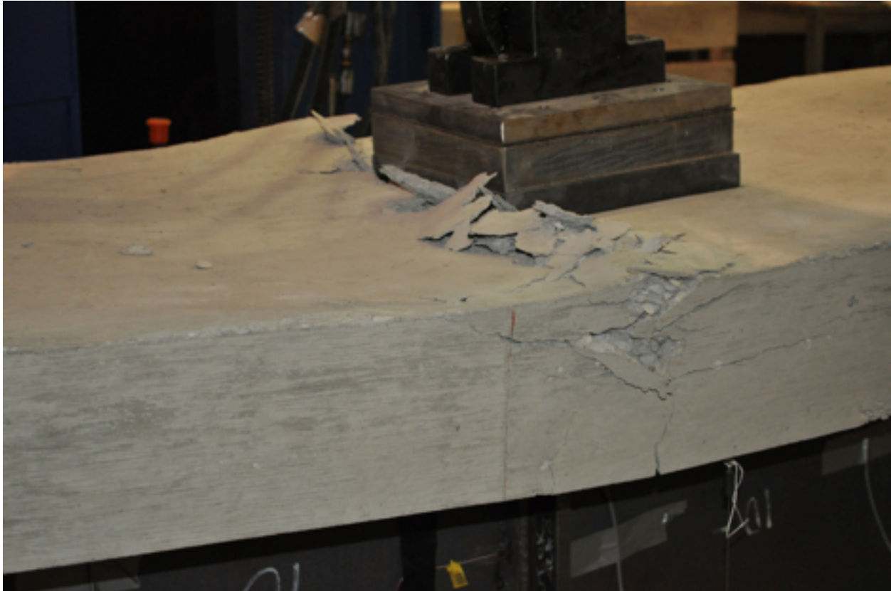
Figure 4.4-9: Concrete deck failure in Specimen 3
