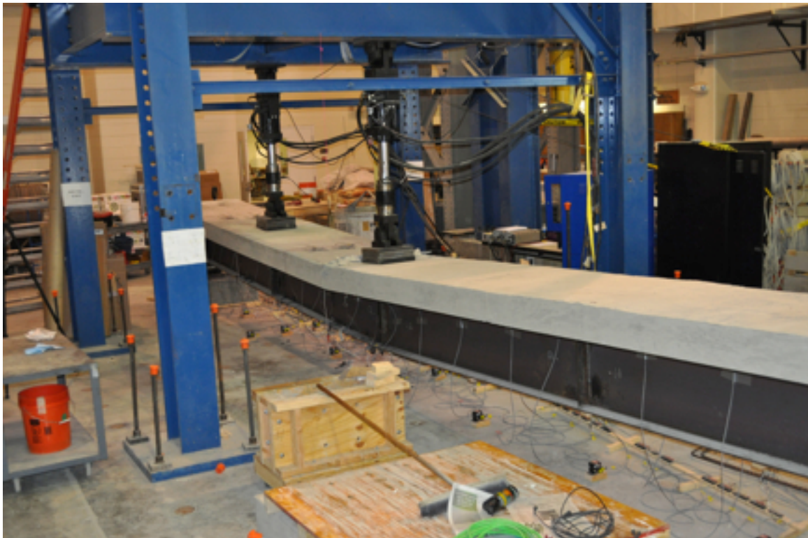
Figure 4.4-7: Deflected shape of Specimen 3 after failure
