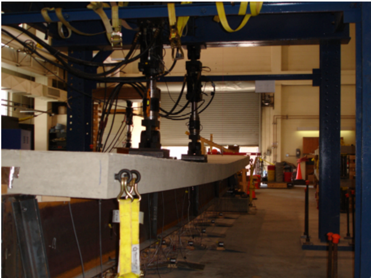
Figure 4.4-2: Deflection of beam specimen under load at midspan and quarterspan
