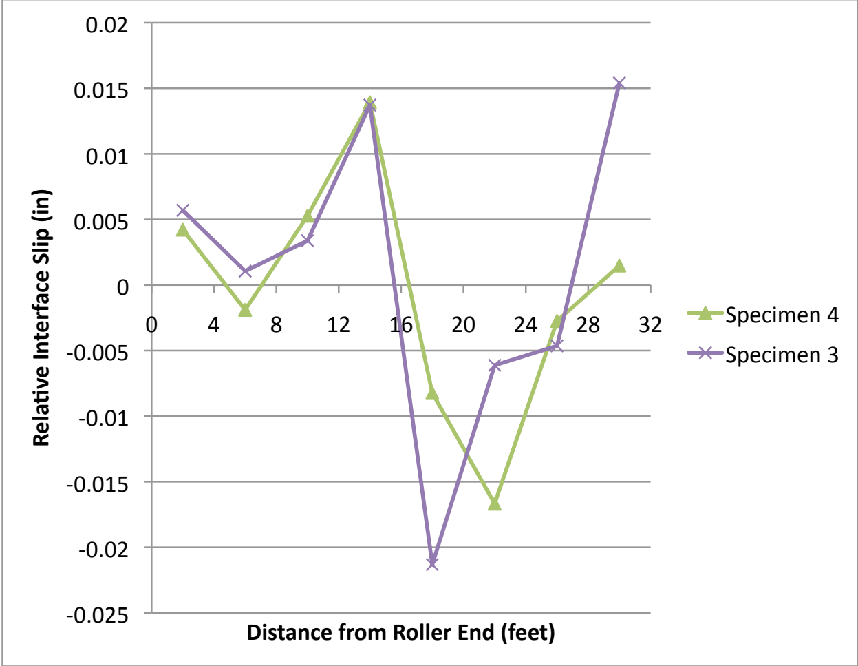
Figure 4.5-8: Plot of Stud Slip vs Distance Along Beam with 70 K at Midspan and Elastic Behavior for Specimens 3 and 4
