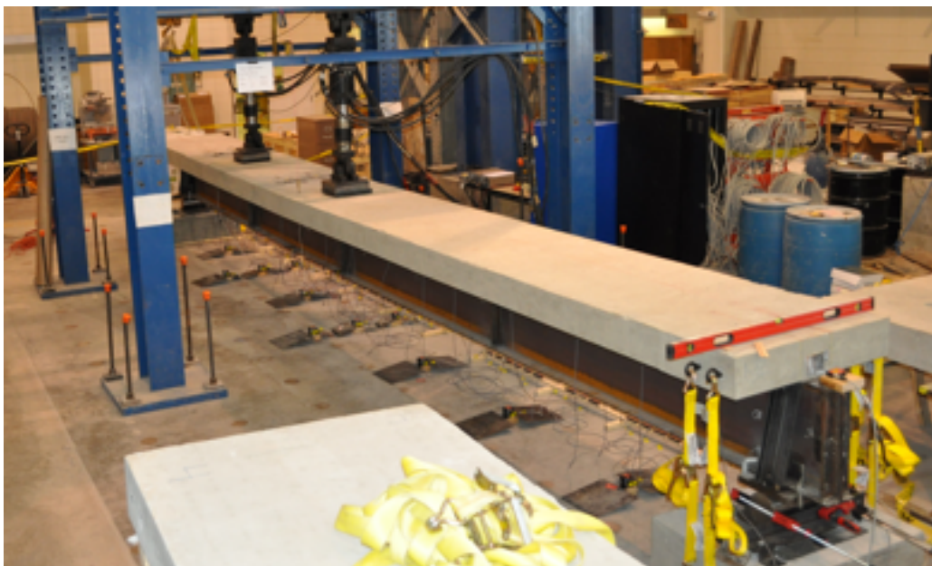
Figure 4.4-1: Beam specimen under load at midspan
