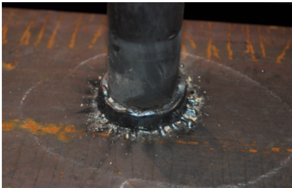
Figure 3.4-2: A typical high quality weld of a large diameter stud on a test specimen
