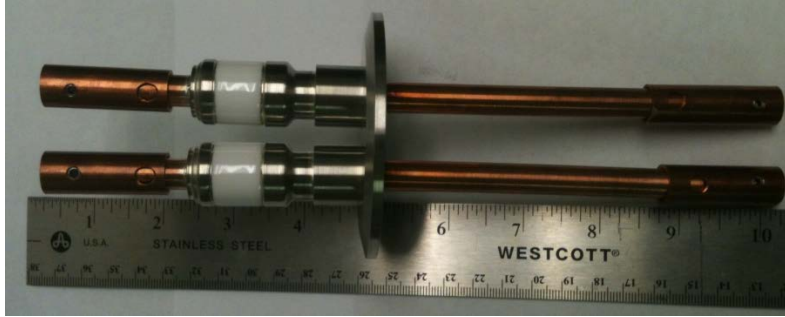
Figure 3-2: High current feed-through used to power the filament source. Copper fittings were made for each lead to connect cables.
