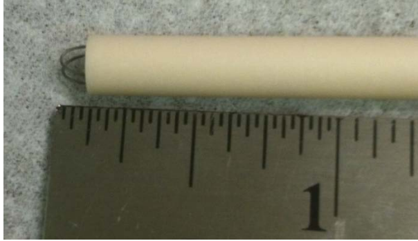
Figure 3-9: Example of the double emissive probe that is used on ALEXIS. Both loops are made from 0.1 mm diameter tungsten wire that has been set in a 3 mm diameter loop.
