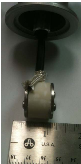
Figure 3-8: A blocking disk is used block out the center of the rf plasma, and to terminate the filament plasma. One side of the disk is biased to the same potential as the stainless steel mesh, so that a uniform plasma potential can be set on the filament plasma.
