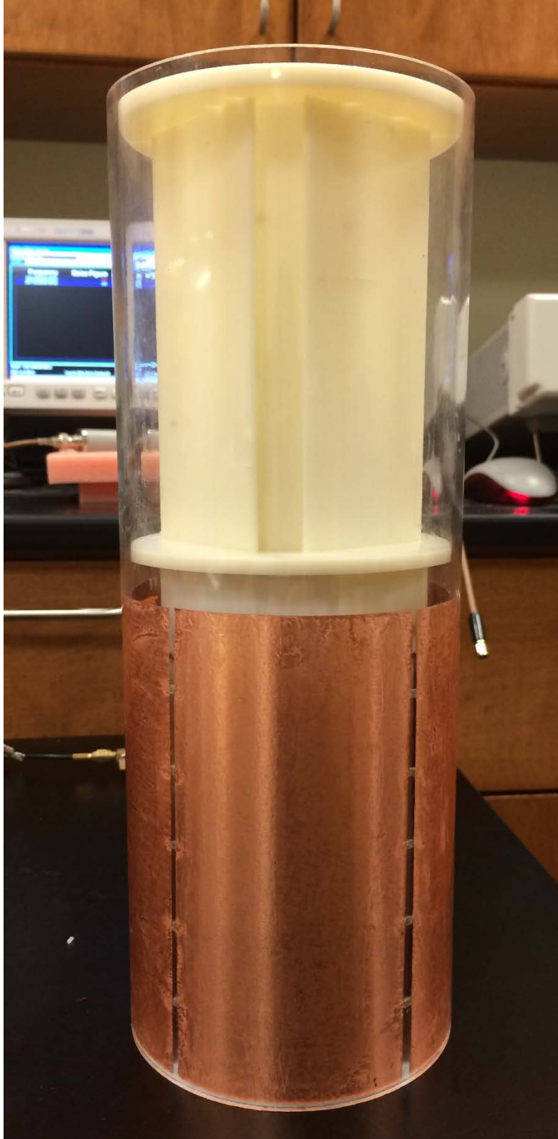
Figure 4.2 Coil Housing Frame Printed out by 3D printer
