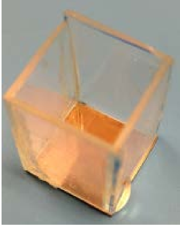
Figure 3.3. Water tight frame for CNT bump fabrication.
