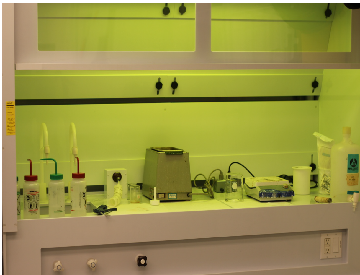
Figure 2.2 Fume hood for sample preparation and cleaning
