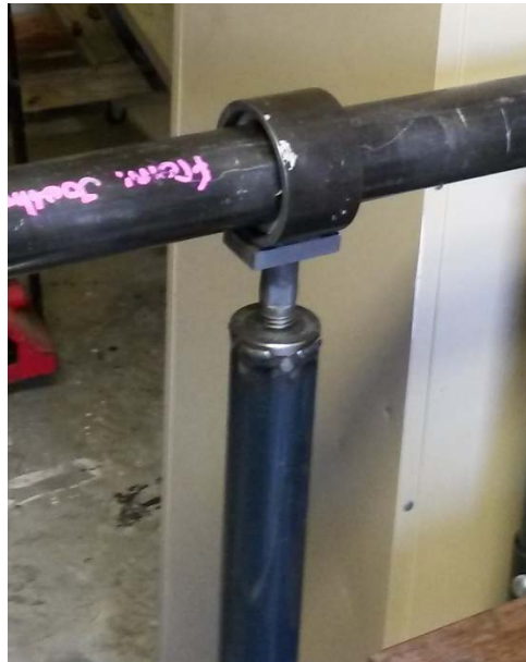
Figure 2.10: Upsized Barrel Delrin Bushing; Center Support
