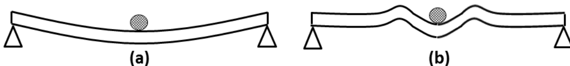
Figure 8.1: Plate Response To (a) Low And (b) High Velocity Impact
