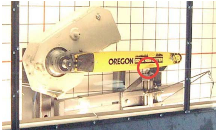
Figure 8.3: Experimental Chainshot Launcher (Skogforsk, 2004)
