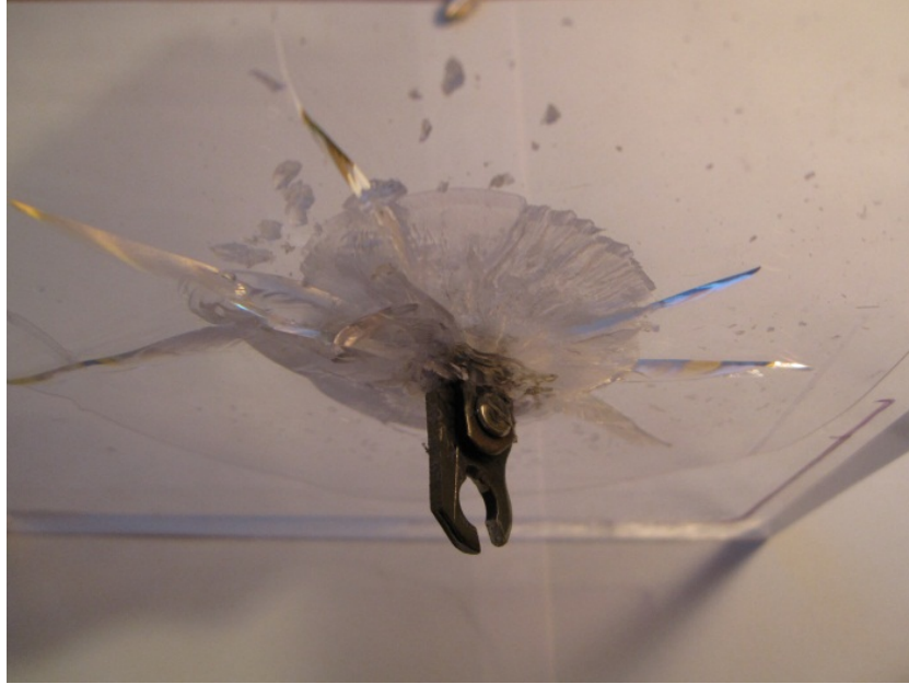
Figure 8.19: 0.75" Laminated Lexan Post-Impact Damage For Test 1; Front Close Up
