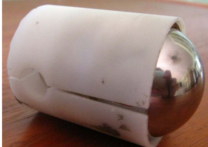
Figure 4.7: Assembled 1-3/8" Spherical Sabot With Projectile
