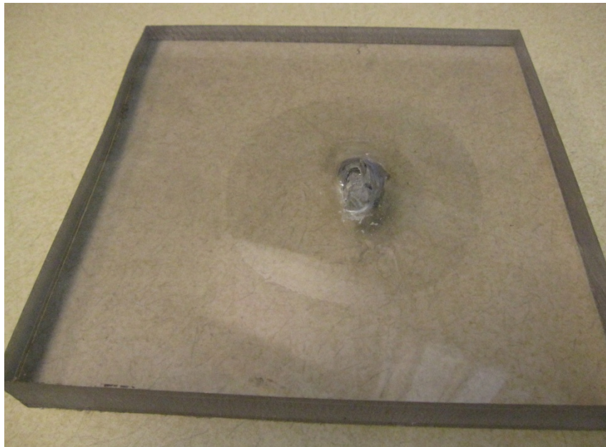
Figure 8.21: 0.75" Laminated Lexan Post-Impact Damage For Test 3; Back
