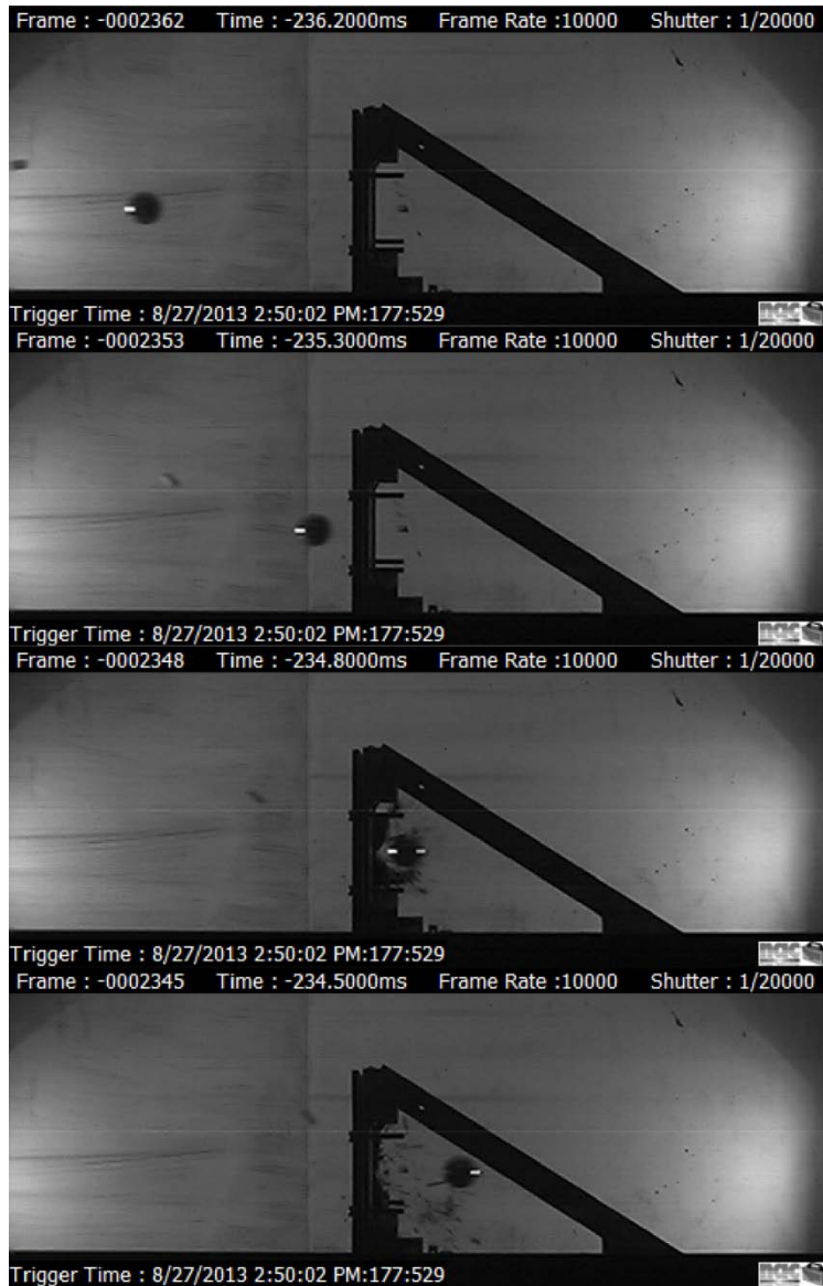
Figure 4.9: High Speed Video Stills Of Large Projectile Sabot Development; 658 fps
