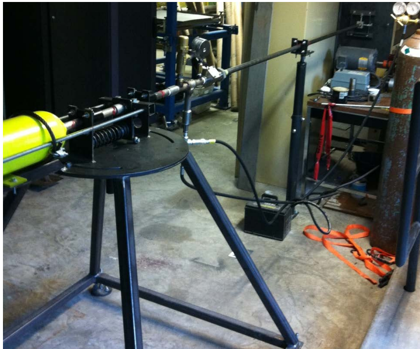
Figure 8.8: Experimental Single-Stage Gas Gun System
