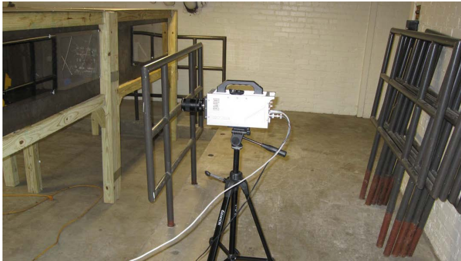
Figure 3.1: High Speed Video Camera Used For Velocity Measurements
