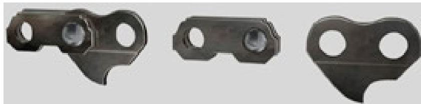
Figure 8.6: Highest Potentially Hazardous Chainshot Fragments (Oregon, 2013)
