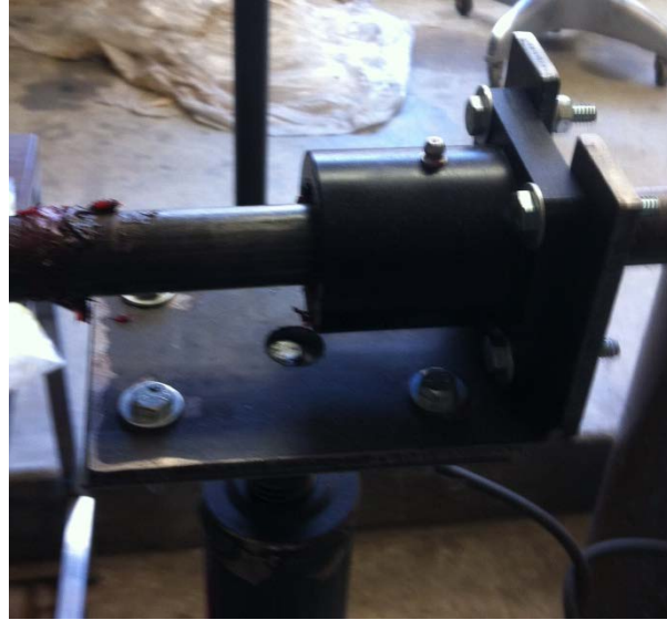
Figure 2.6: Barrel Center Support With Linear Bearing
