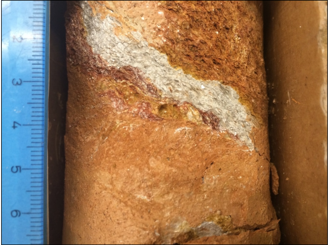
Figure 37: Short section of drill-core 09-02. Depth is 2.14 m. Saprolitic, foliated muscovite schist. Note small inconsistent phacoids in foliation dipping at 80°; direction of dip unknown. Scale is in cm on the left.
