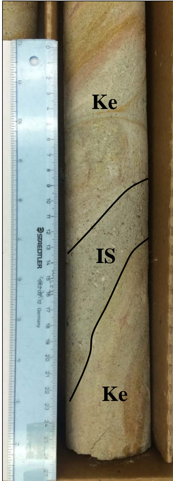
Figure 34: Short section of drill-core 09-02. Depth is 18.23 m. Note the fine-grained Eutaw Formation unit (Ke) surrounding impactite-sand injection (IS). Eutaw sands appear to be folded and deformed to accommodate the dike injection. Scale is in cm and inches on the left.
