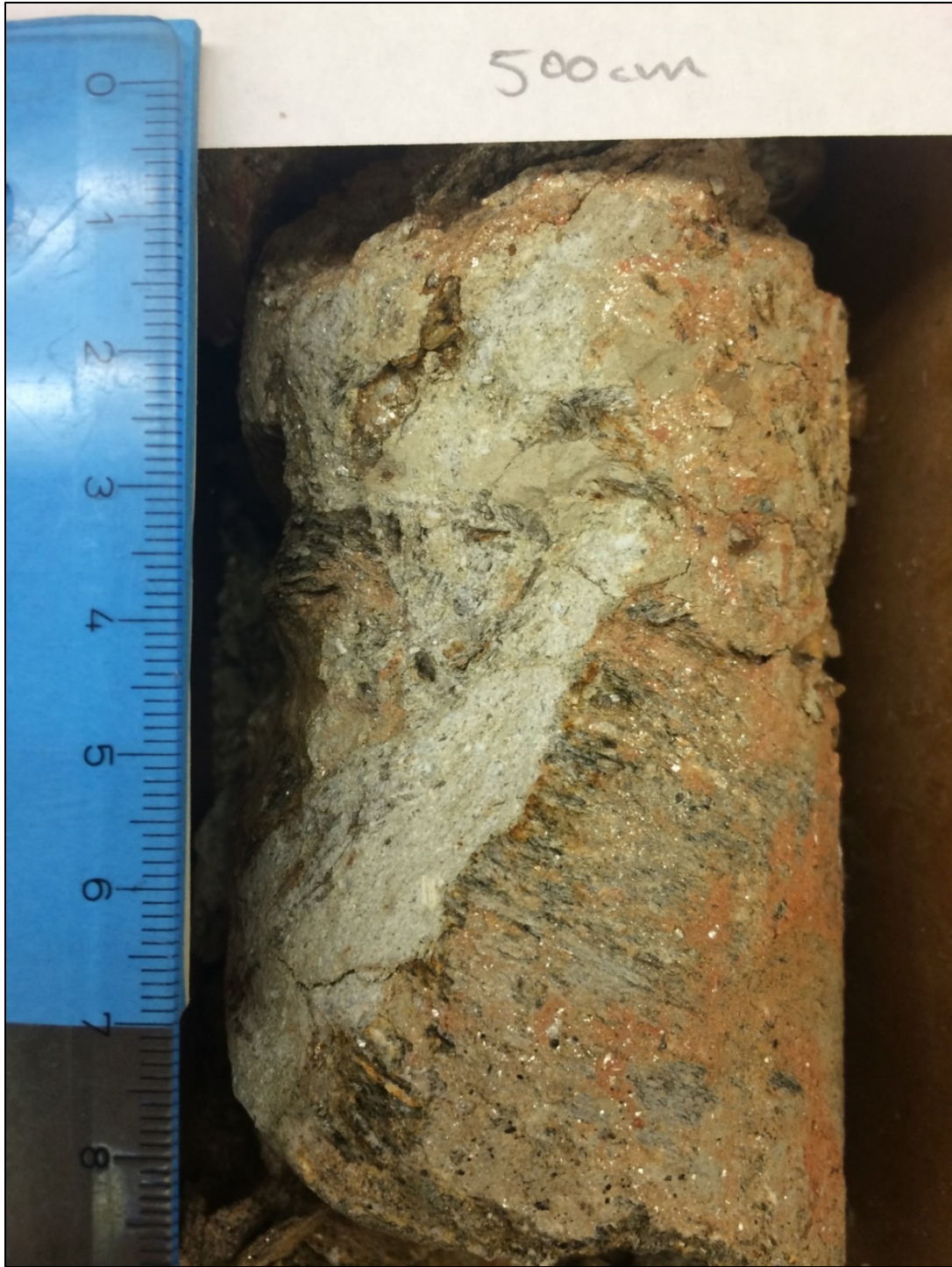
Figure 33: Short section of drill-core 09-02. Depth is 5 m. Note fine grained impactite sand injection (left) cross cutting weathered gneiss (right). Centimeter scale on left.
