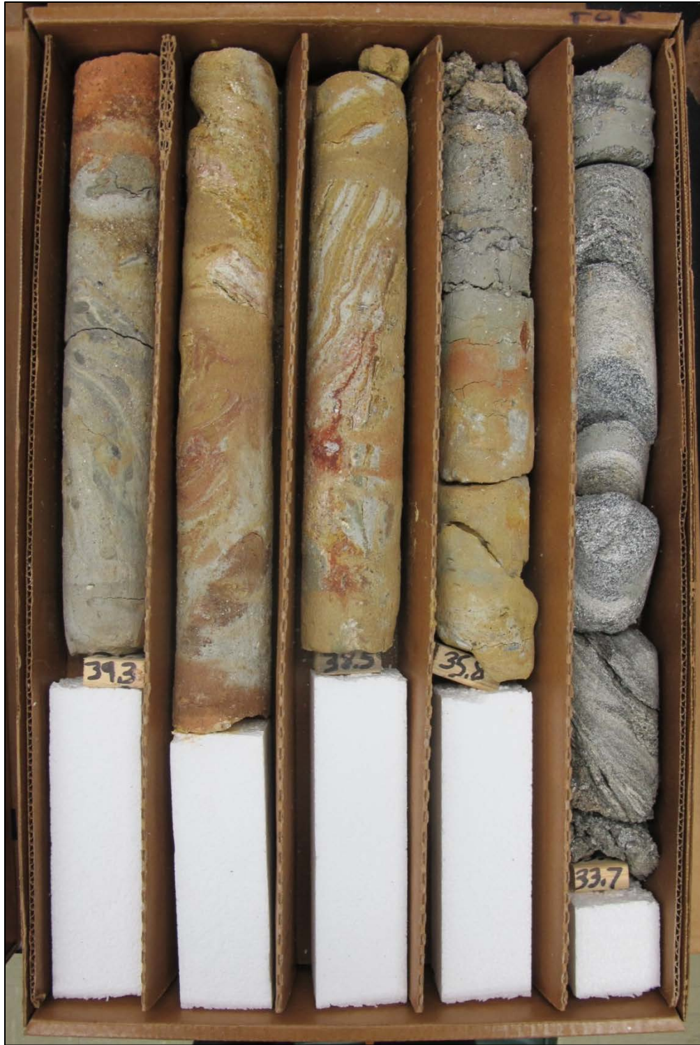
Figure A6: Photograph of drill-core 09-02, box 4 (9.60 m – 11.98 m). Up is top right; bottom is lower left. Wood depth marker is in feet.
