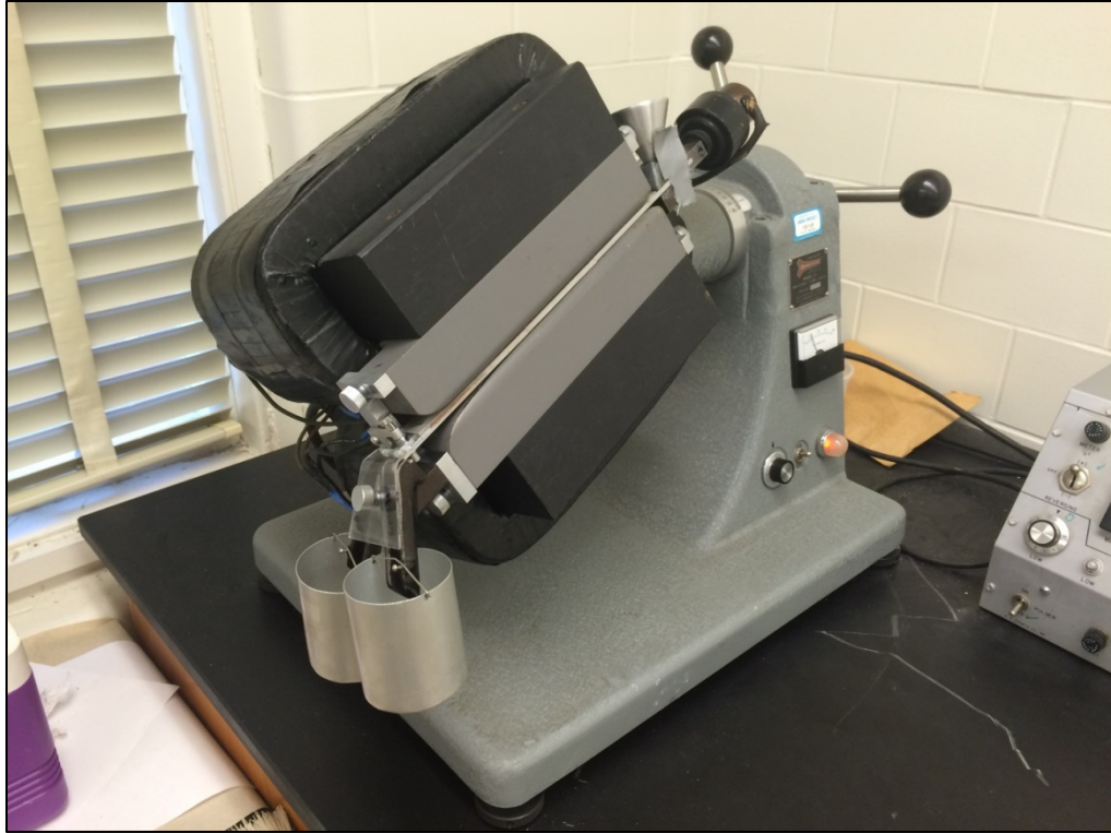
Figure 10: Photograph of the Frantz Isodynamic Magnetic Separator used for heavy mineral separation.
