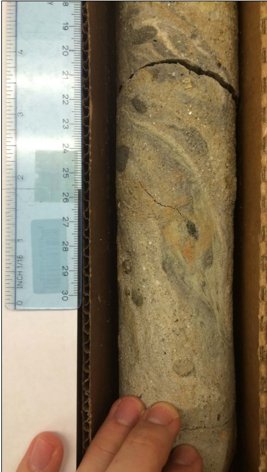
Figure 35: Short section of drill-core 09-02. Depth is 11.77 m. Note flow textured structures within coarser grained impactite sand (left). Scale is in cm and inches on the left.
