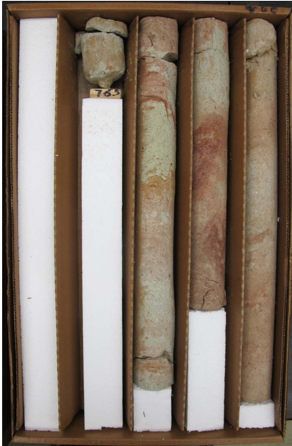
Figure A10: Photograph of drill-core 09-02, box 8 (21.79 m – 23.32 m). Up is top right; bottom is lower left. Wood depth marker is in feet.
