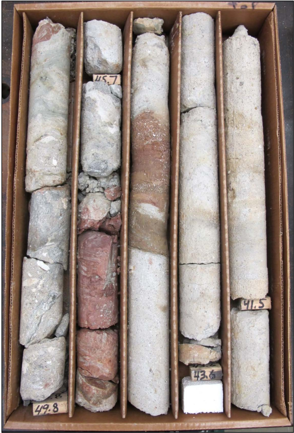
Figure A7: Photograph of drill-core 09-02, box 5 (11.98 m – 15.16 m). Up is top right; bottom is lower left. Wood depth marker is in feet.
