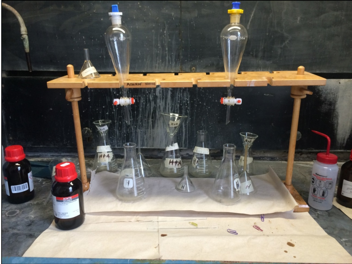
Figure 9: Photograph of the heavy-mineral extraction set up used in this study.
