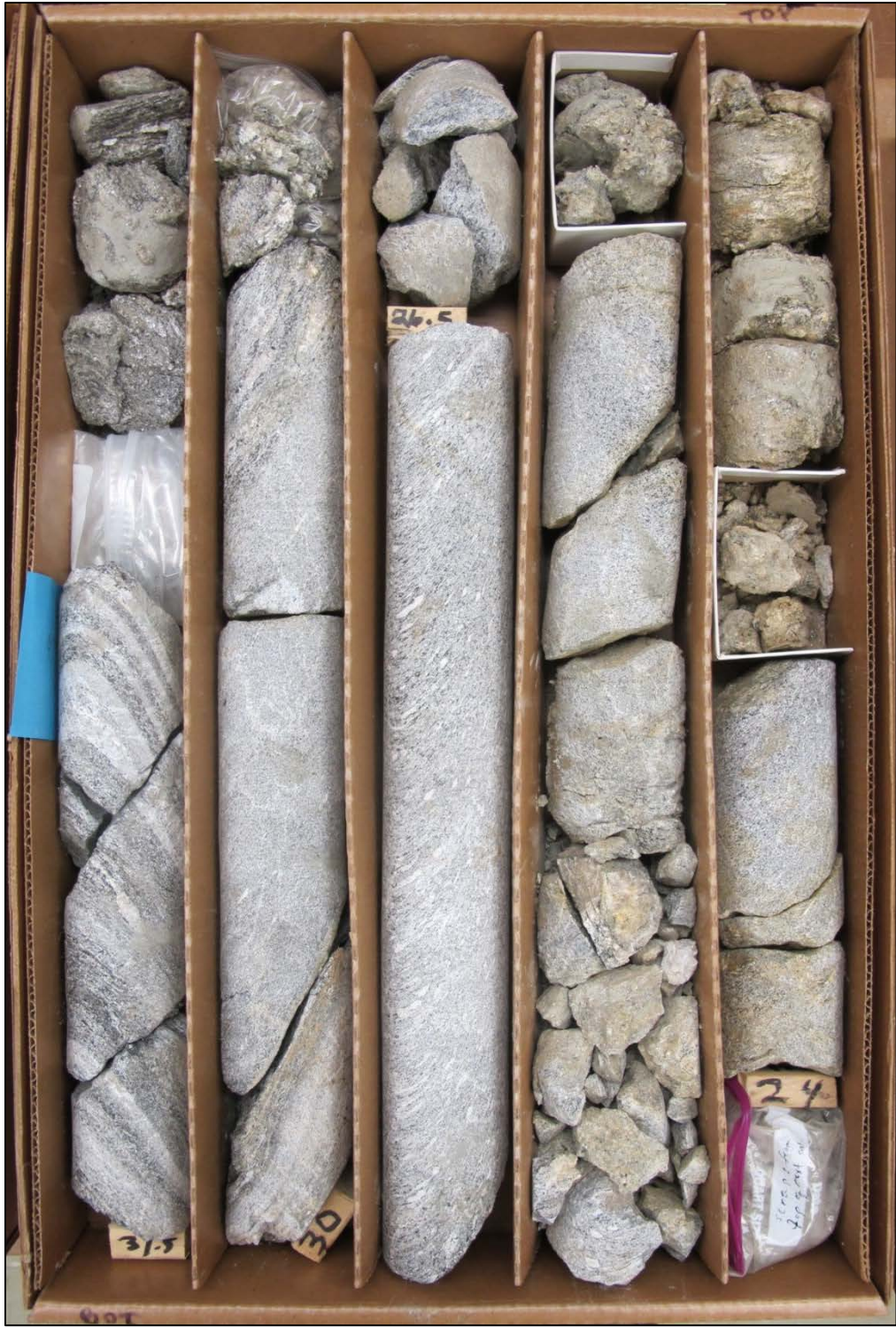
Figure A5: Photograph of drill-core 09-02, box 3 (5.99 m – 9.60 m). Up is top right; bottom is lower left. Wood depth marker is in feet.
