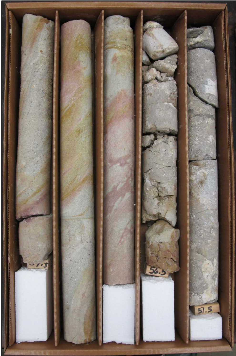
Figure A8: Photograph of drill-core 09-02, box 6 (15.18 m – 18.75 m). Up is top right; bottom is lower left. Wood depth marker is in feet.
