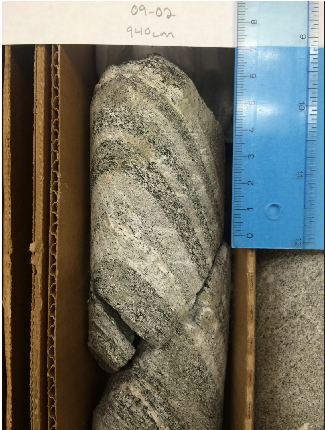
Figure A1: Short section of drill-core 09-02. Depth is 940 cm (9.4 m). Note banded augen (feldspar clast) gneiss. “V” folds dipping 48^\circ in an unknown direction. Up is at the top of the photograph. Scale is in cm and inches on the right side.
