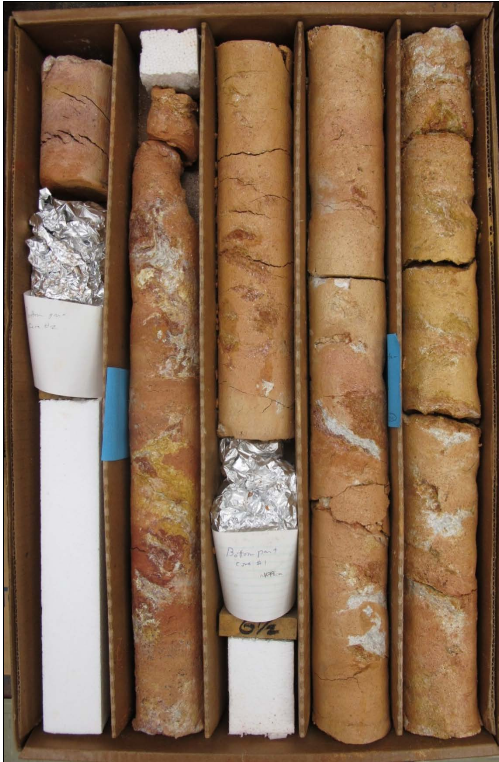
Figure A3: Photograph of drill-core 09-02, box 1 (0.457 m – 3.51 m). Up is top right; bottom is lower left. Wood depth marker is in feet.
