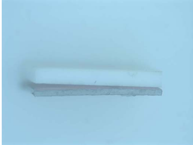
Figure 2-25 Cu foil delamination after 250 thermal cycles
