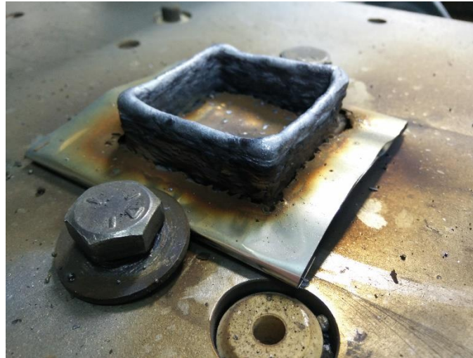
Figure 99: Steel (ER70S-6) Deposited on Chrome Alloy Foil
