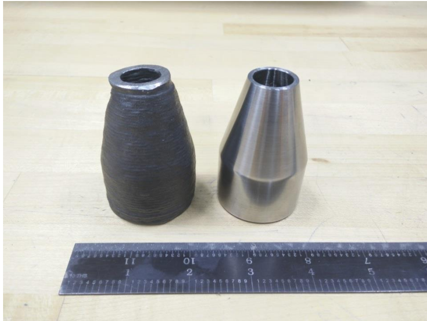
Figure 66: Stainless Steel (ER308) Nozzles
