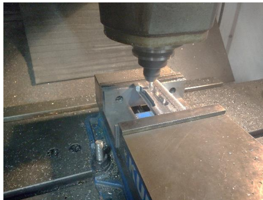
Figure 50: CNC Mill Machining Tensile Test Specimen
