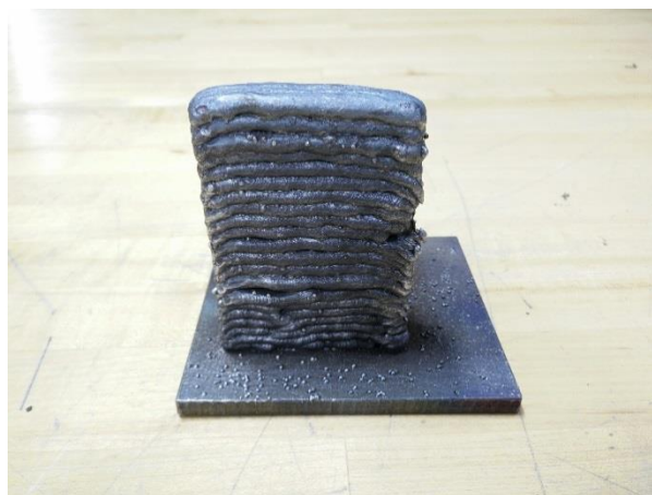
Figure 56: Heat Treatment Test Specimen before Cutting
