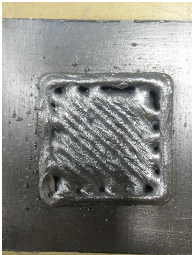
Figure 63: Straight Solid Infill in Steel (ER70S-6)
