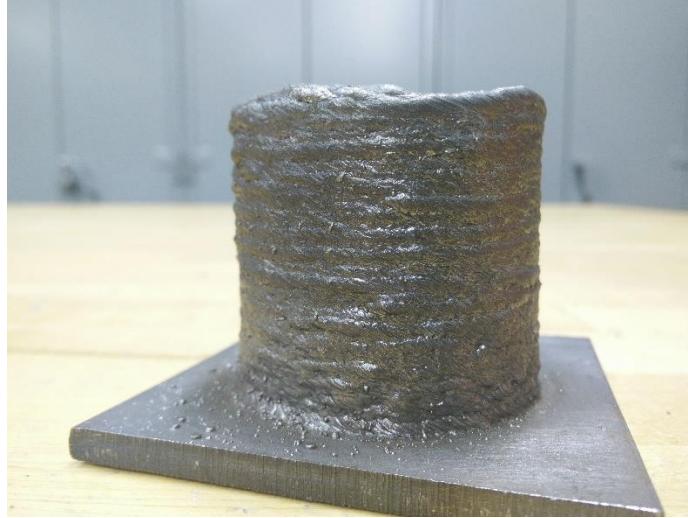
Figure 60: Cylinder with Randomized Layer Start Points in Steel (ER70S-6)
