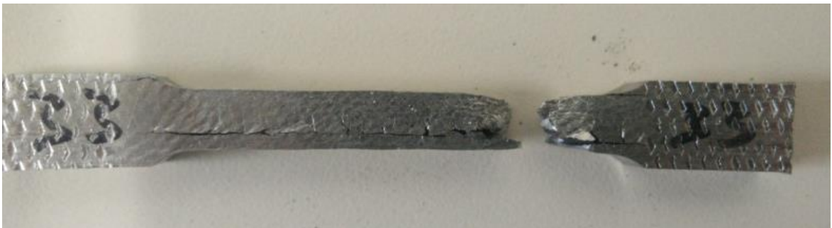
Figure 70: Steel (ER70S-6) Horizontal Tensile Specimen Failure
