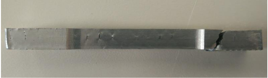
Figure 73: Steel (ER70S-6) Vertical Tensile Specimen Failure
