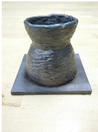
Figure 65: Hourglass Shape in Steel (ER70S-6)
