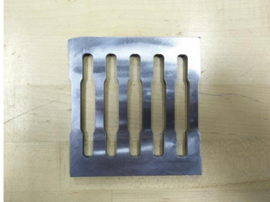
Figure 51: Tensile Test Specimens after CNC Machining
