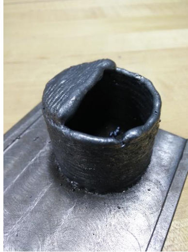
Figure 64: Overhanging Wall in Steel (ER70S-6)
