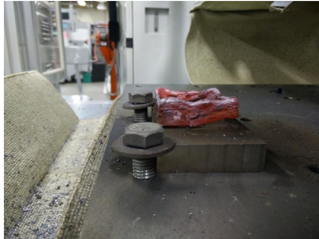
Figure 97: Steel (ER70S-6) Cooling on Titanium Build Plate
