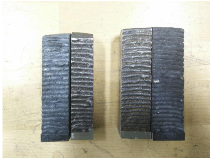
Figure 57: Separated Heat Treatment Test Wall Structures
