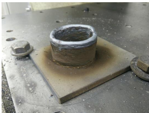
Figure 45: Steel Wire (ER70S-6) Diameter Study Specimen
