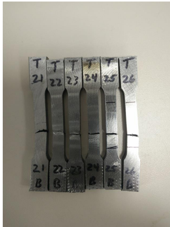
Figure 76: Broken Steel (ER70S-6) Tensile Specimens from Wall 2
