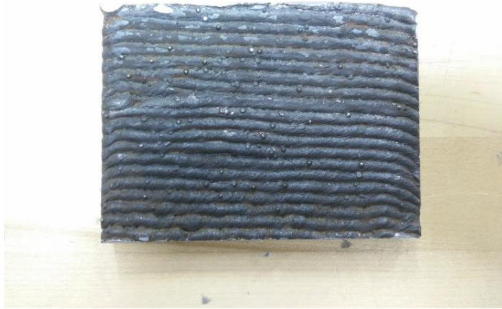
Figure 49: Machined Square Tensile Test Specimen Wall
