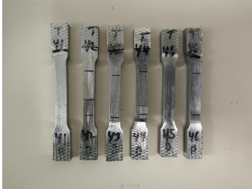
Figure 77: Broken Steel (ER70S-6) Tensile Specimens from Wall 4
