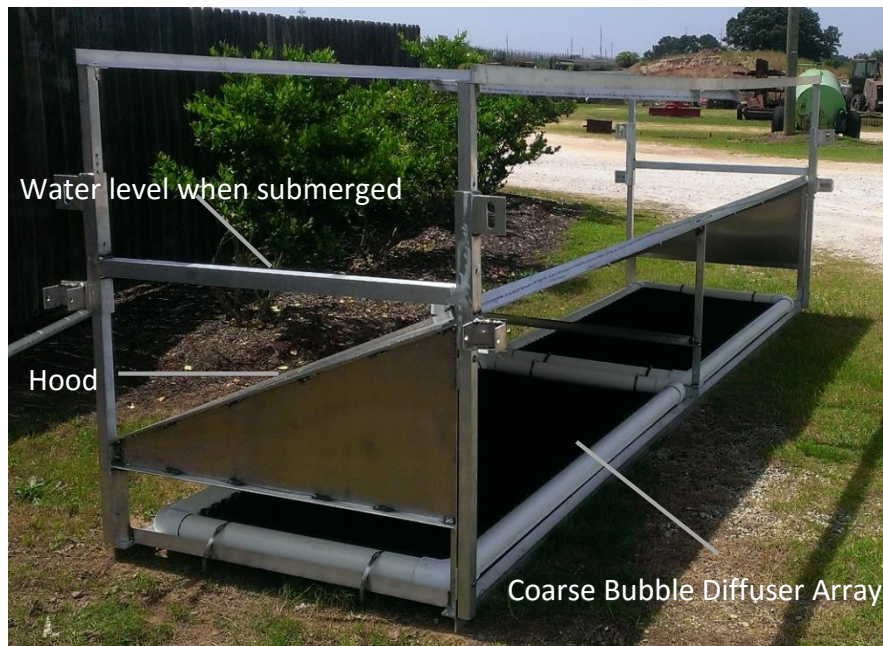
Figure 3.10 Five meter long diffused air hood out of water (shown without floats).
