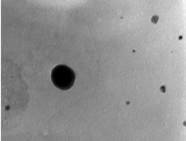
Figure 3. A representative transmission electron microphotograph of nanoparticles prepared with maltodextrin and trimesoyl chloride. The sample is dry-mounted on a copper grid coated with polyvinyl alcohol film. Magnification was (a) 100,000 (b)160,000.
