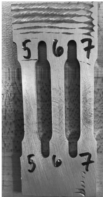
Figure 142. Tensile specimen as-machined and a table of the measured sizes. Note that the specimens shown are transverse specimens 1, 2, and 3 and are incorrectly labeled.
