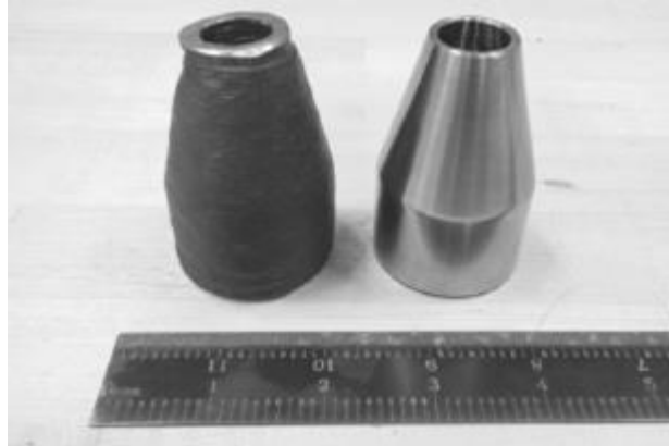
Figure 30. Stainless steel nozzle as-printed and post-machining [4]
