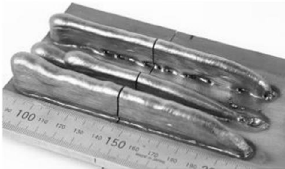
Figure 63. Walls showing the changing bead geometry at the start and end of weld [44]
