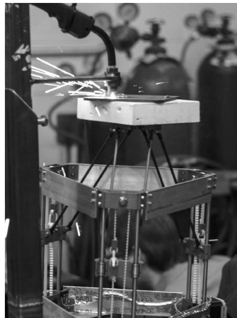
Figure 27. Sprocket made via the low-cost open-source MIG printer by Anzalone [35]
