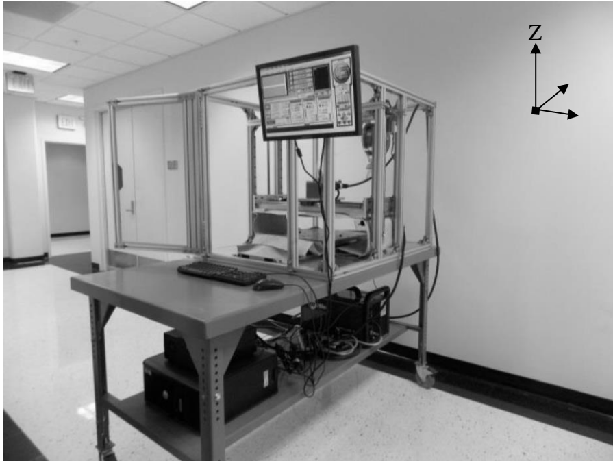
Figure 68. Gantry CNC machine used as base for WAAM research [4]
