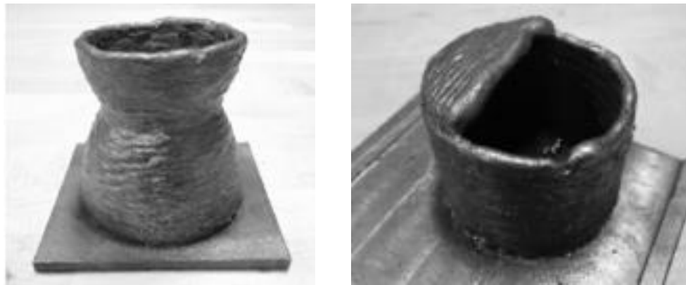
Figure 29. Outward and inward facing geometry test (left) and bridging test (right) [4]
