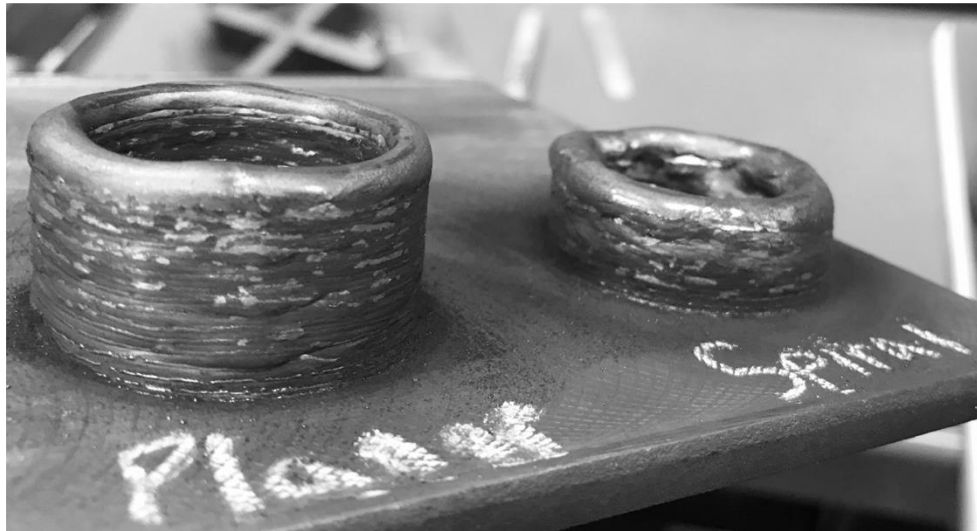
Figure 93. ER70S-6 single-bead cylinders made with the spiral method (right) and layer-by-layer method (left)
