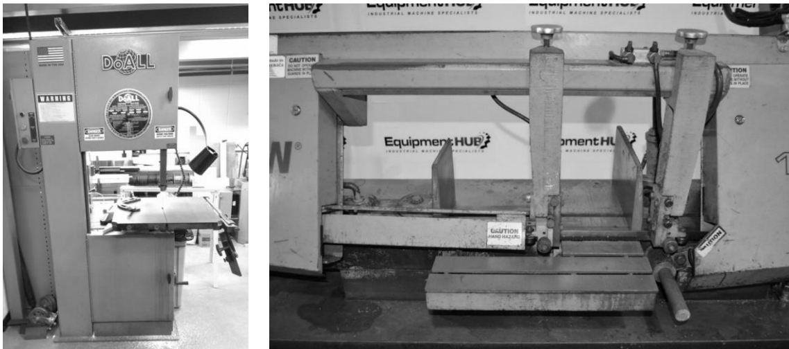
Figure 80. Do-All 2013-V Vertical Band Saw (left) and the Wellsaw 1118 Horizontal Band Saw (right)
