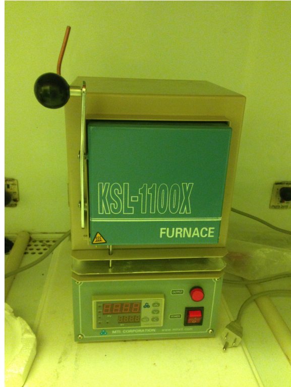
Figure 2.4: Annealing furnace KSL-1100X.
