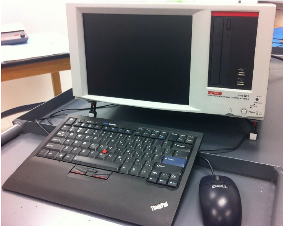
Figure 2.27: Keithley 4200 (Semiconductor Characterization Systems) parameter analyzer.
