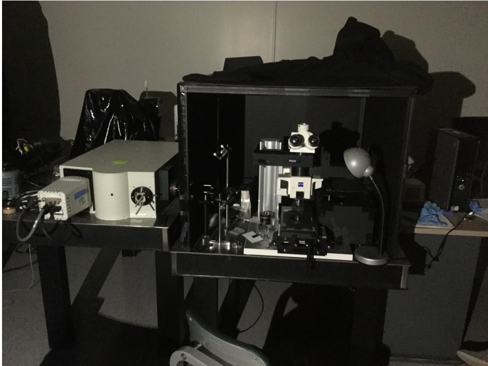
Figure 2.22: Home-made Raman spectroscopy and photoluminescence (PL) system.
