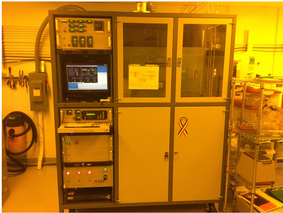
Figure 2.15: Low pressure chemical vapor deposition (LPCVD) system.
