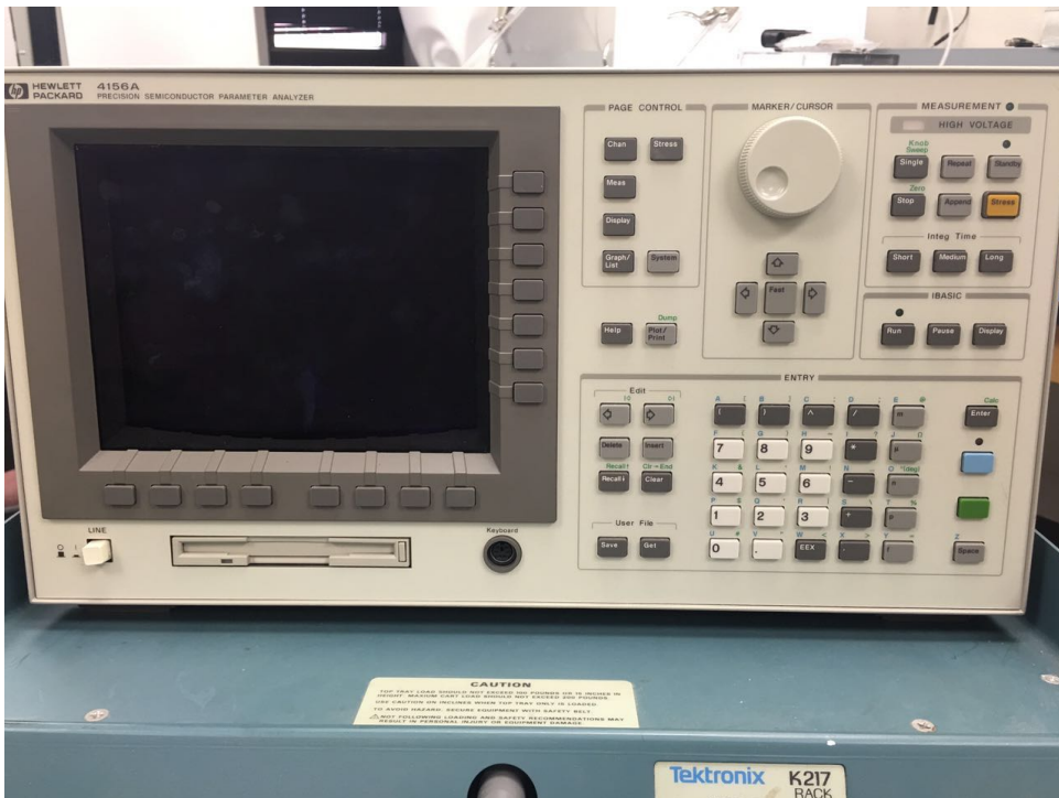
Figure 2.28: HP 4156 A (Semiconductor Characterization Systems) parameter analyzer.
