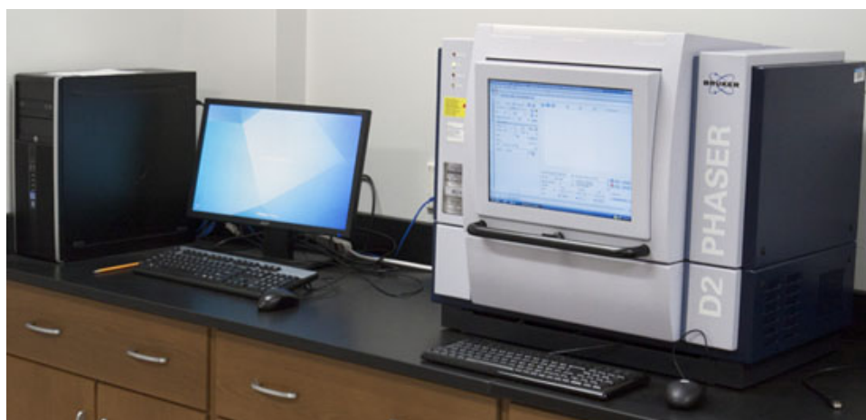
Figure 2.23: Bruker D2 Phaser X-ray diffractometer.
