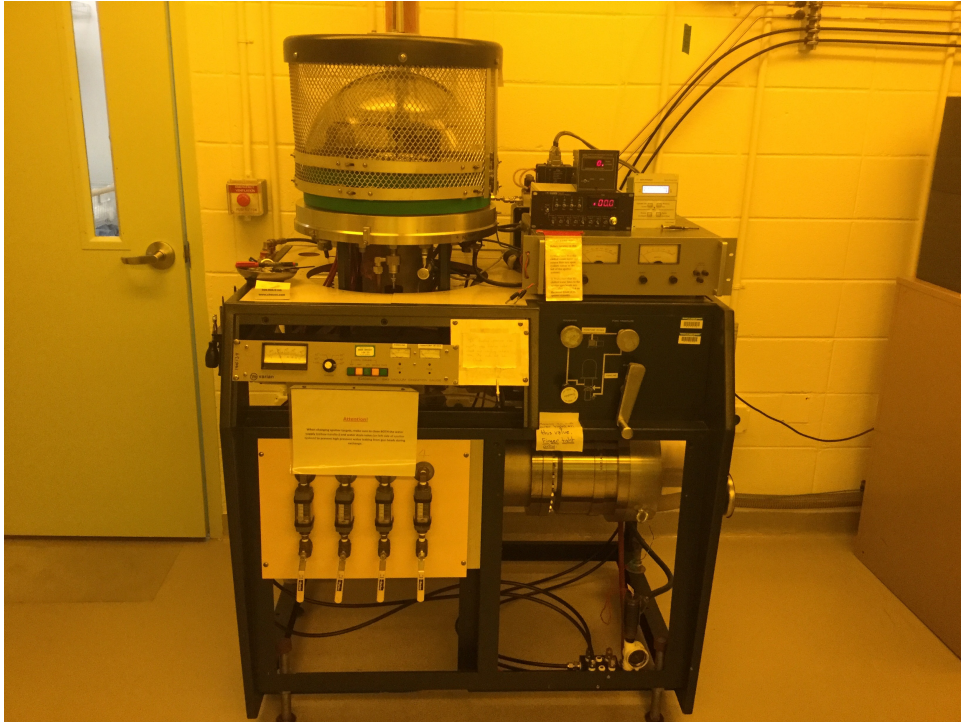
Figure 2.11: Direct current (DC) magnetron sputtering system.
