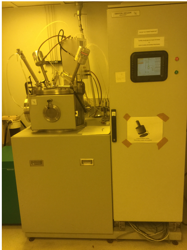
Figure 2.5: RF magnetron sputtering system.
