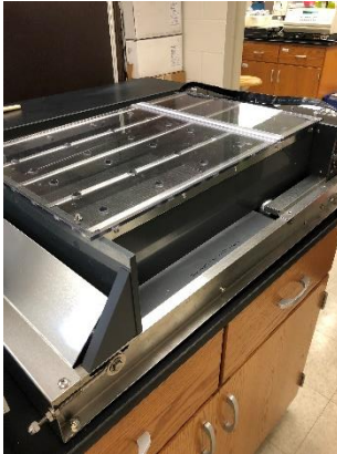
Figure 20. Rodent Treadmill. An exercise treadmill designed specifically for biomedical and kinesiology research using rodent models was used for metabolic heat stress experiments. In this forced exercise model, animals were placed on an active treadmill for 25 minutes. Rectal temperature was taken before and after exercise-induced stress, and biochemical parameters and EOG recordings were assessed after 4 hours.
