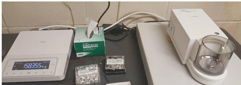
Figure 18: Microbalance for algal biomass determination. (range: 3 mg., resolution: 1 ug)
