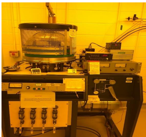
Figure 3.5. The dc-magnetron sputtering system used for the metal deposition in this research.
