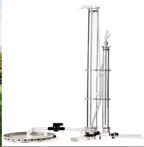
(b) Disk infiltrometer.
