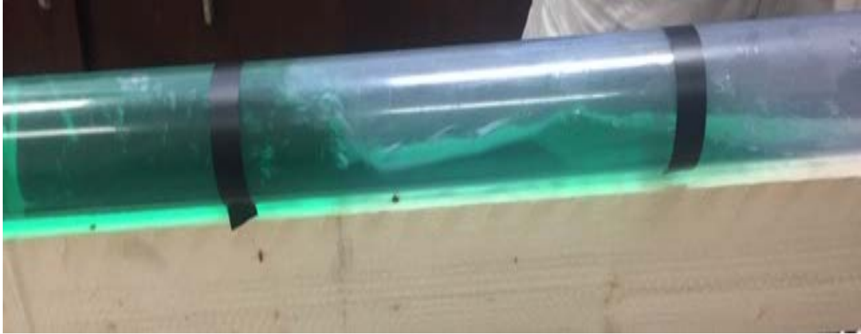
Figure 5. 11. Typical early stage air-water interface for 10 degree slope and A_v^* = 0.035 , A_o^* = 0.25 prior to becoming near horizontal
