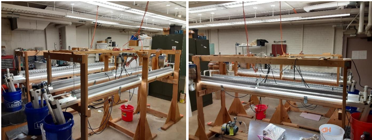
Figure 3.4. Pictures of the indoor ATS system used in the experiment, left to right: the four lanes used in the experiment and a side view of an individual lane.
