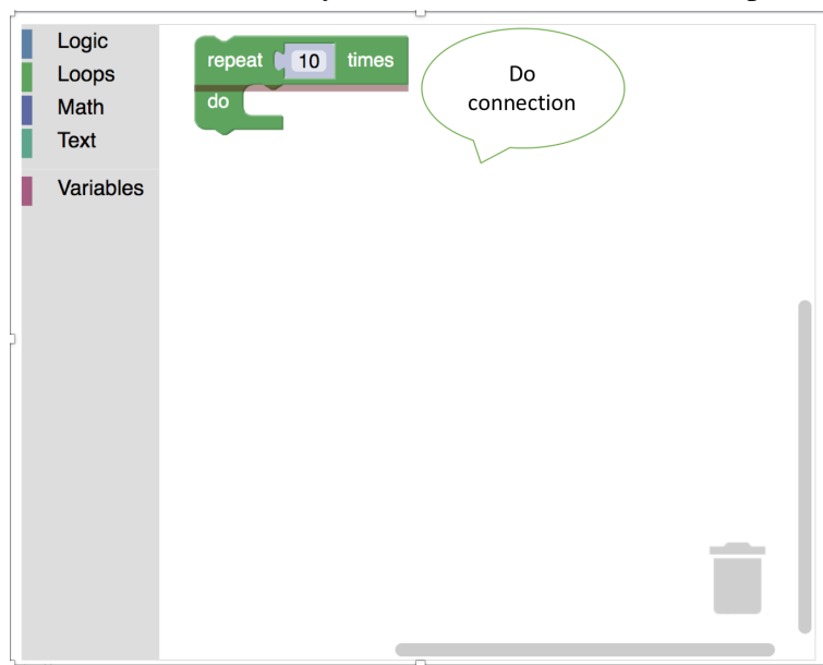
Figure 4.3: A Blockly environment with a repeat 10 times block on its workspace. The do connection is illustrated with a red line.
