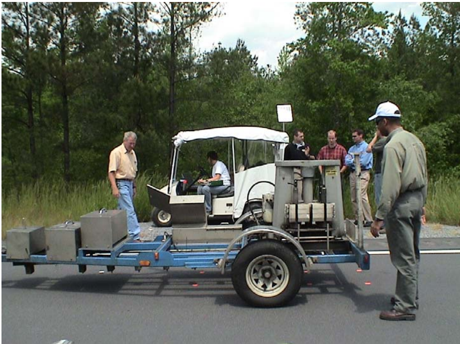
Figure 3.8. FWD Testing and Data Collection.
