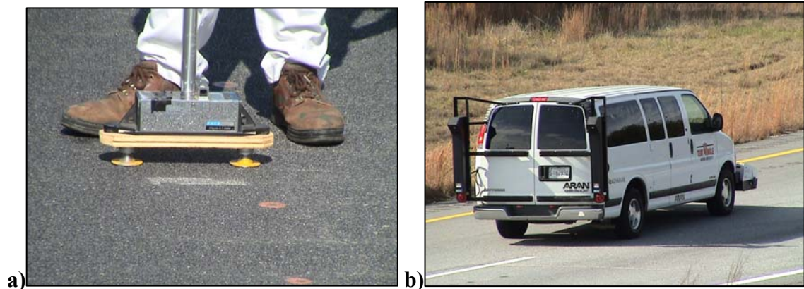
Figure 3.12. Rut Depth Measurements a) Dipstick b) Automated Pavement Survey Vehicle.
