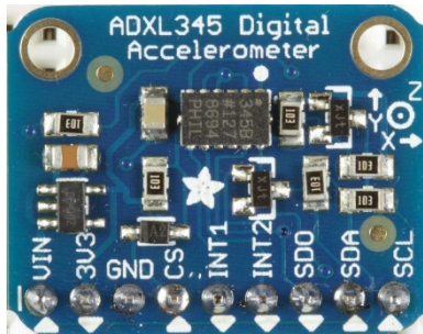
Figure 4.2 ADXL 345 accelerometer sensor and Raspberry pi
