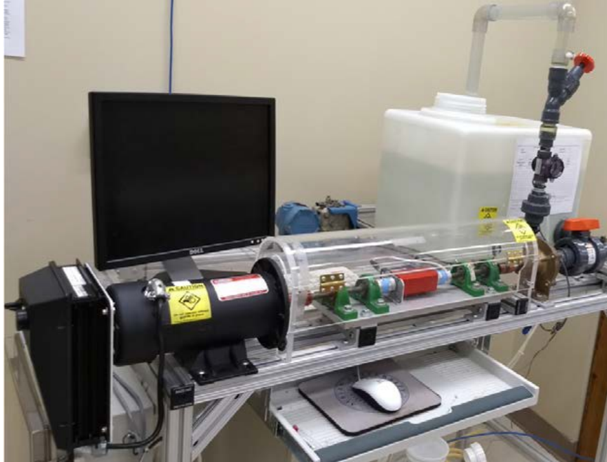
Figure 4.1 Multi stage centrifugal pump setup
