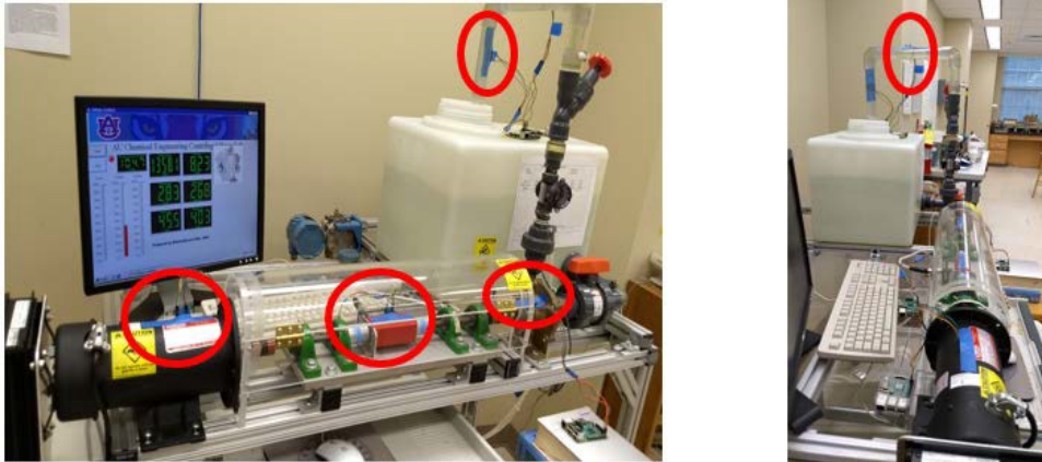
Figure 4.3 IIoT enabled centrifugal pump testbed (Sensors are marked in red)
