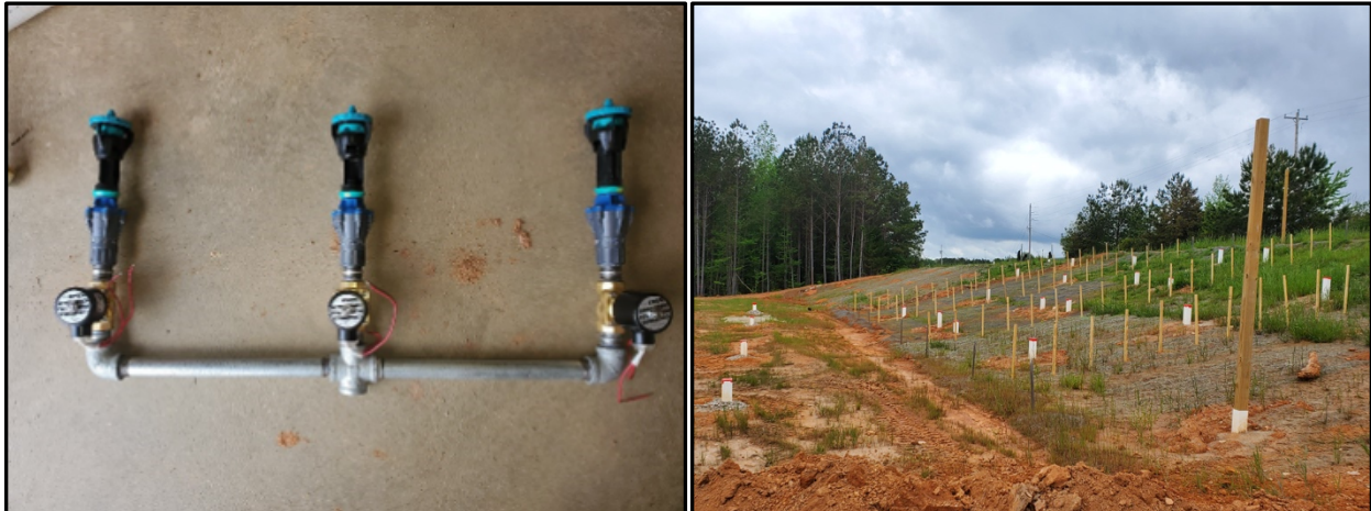
(a) Sprinkler head assembly
