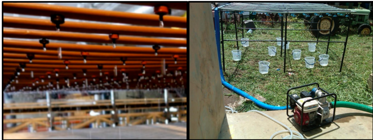
(a) Drip forming rainfall simulator (Naves et. al 2020)
