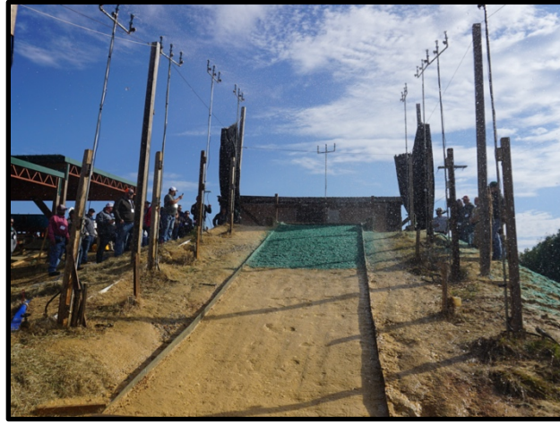
FIGURE 2.4: Existing ASTM D6459 Rainfall Simulator at the Auburn Stormwater Research Facility (Wes Donald)
