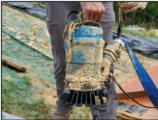
(a) Hydromulch residue on pump (ProMatrix™)
