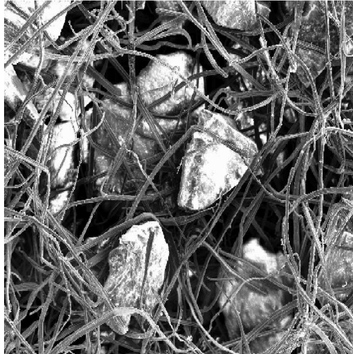
Figure I-11. \gamma -Al 2 O 3 particles entrapped in the matrix of 8 \mu m Ni fibers. SEM was provided by CM 3 .
