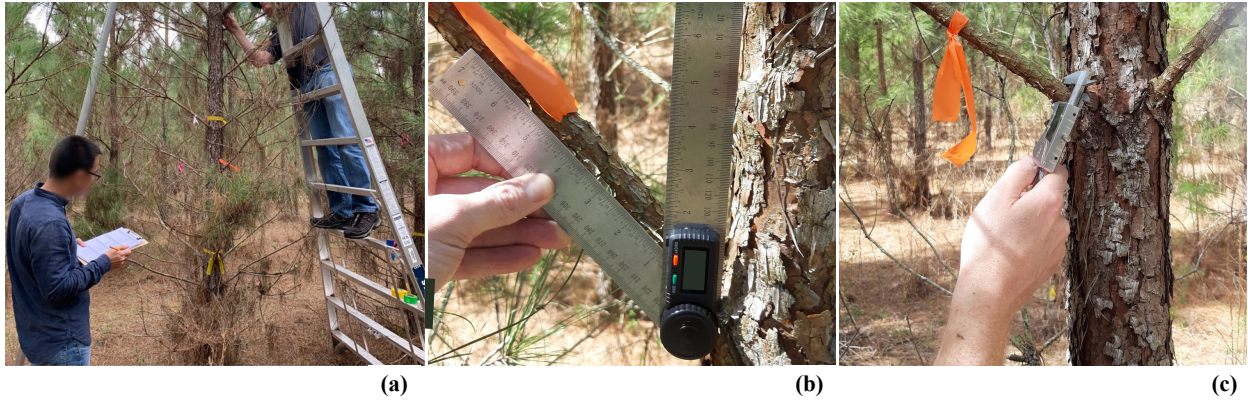
Figure 3-1. (a) In-field acquisition of ground-truth data: (a) 1 m intervals up to a height of 5m were demarcated on the stem using flagging tape, and the stem diameter at each meter interval was measured using a diameter tape, (b) A digital angle finder was used to measure branch angle relative to the vertical stem, and (c) a digital caliper was used to determine branch diameter adjacent to the stem.
