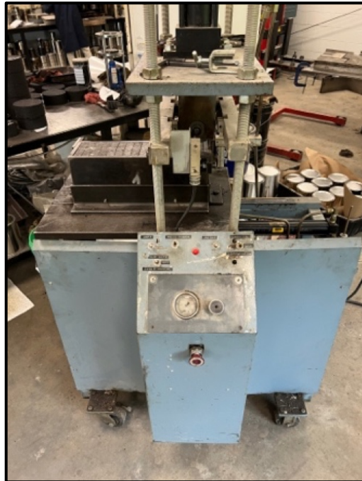
Figure 3.7.1: Beam Fatigue Specimen Compactor
