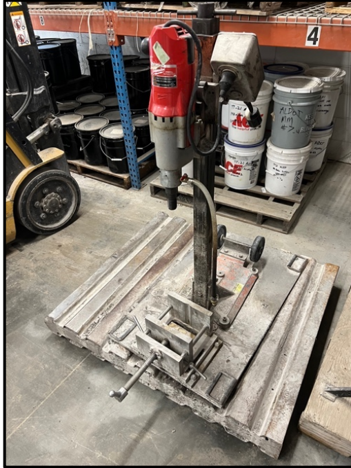
Figure 3.4.3: Small Specimen Core Drill
