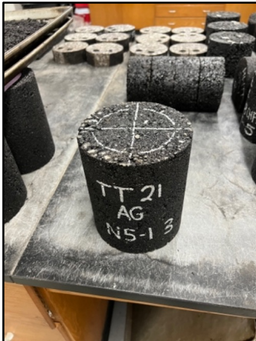
Figure 3.4.2: SGC Specimen with Coring Guide Markings
