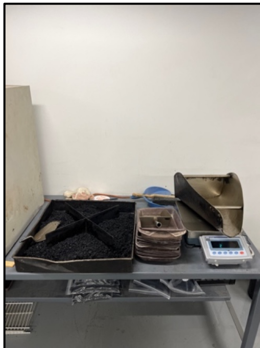
Figure 3.3.3: Specimen Quartering and Reduction
