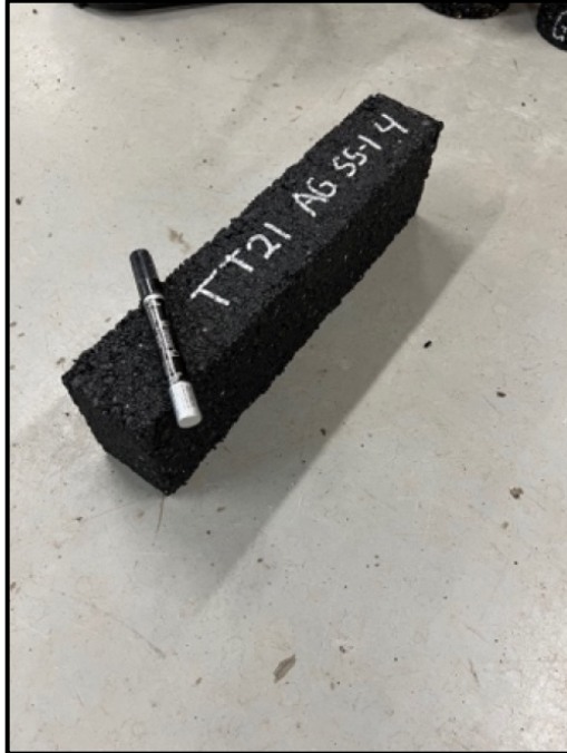
Figure 3.7.2: Compacted Beam Fatigue Specimen
