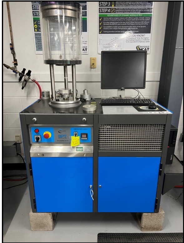
Figure 3.5.1: IPC Global ® AMPT Used for E* Testing
