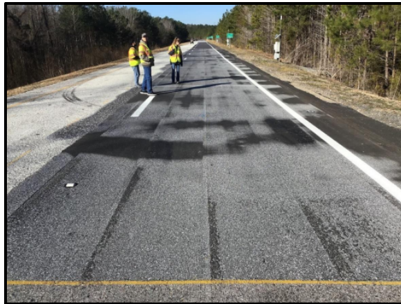
Figure 5.2.1: Example AG Test Section After Precision Grinding (Foshee, 2022)
