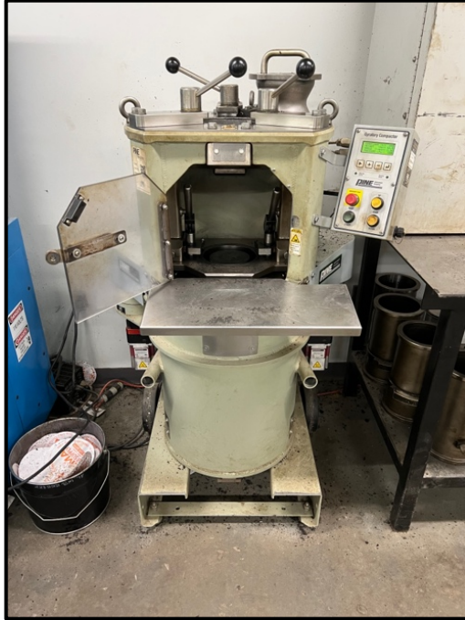
Figure 3.4.1: Superpave Gyrotory Compactor
