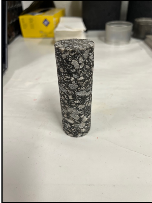
Figure 3.4.5: Example of Final Small Cylindrical Performance Test Specimen
