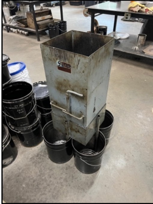
Figure 3.3.2: Sample Splitting with Type A Mechanical Splitter
