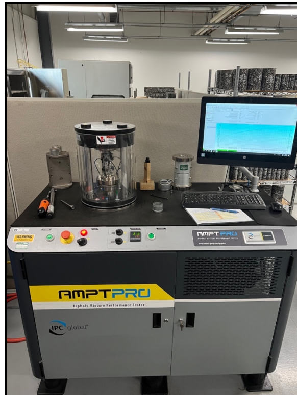
Figure 3.6.1: IPC Global ® AMPT Pro Used for Cyclic Fatigue Testing
