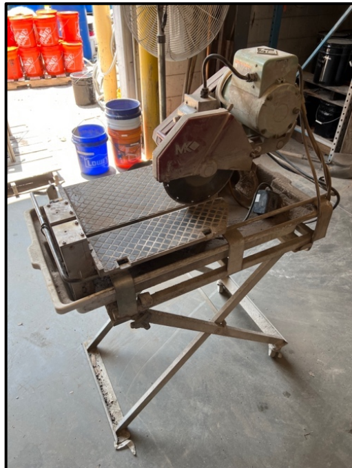
Figure 3.4.4: Small Specimen Wet Saw
