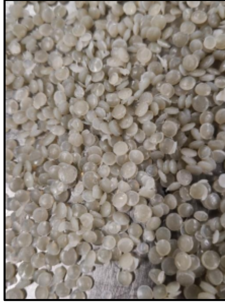
Figure 2.1.5: Typical Dry-Process rPE Additives (Yin, 2022)
