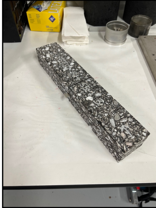
Figure 3.7.4: Example of Final Beam Fatigue Test Specimen
