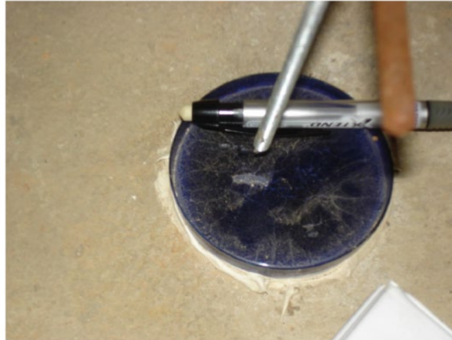
Figure 2-9. Wax plate for tracking the motion of the bridge (Davidson et al., 2012)
