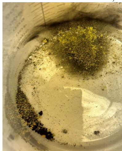
Figure 4.17: an image of residuals from a fire occurred during Ir source refilling.
