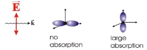
Figure 3.30: An example of search light effect in K-edge. (Adapted from [123])
