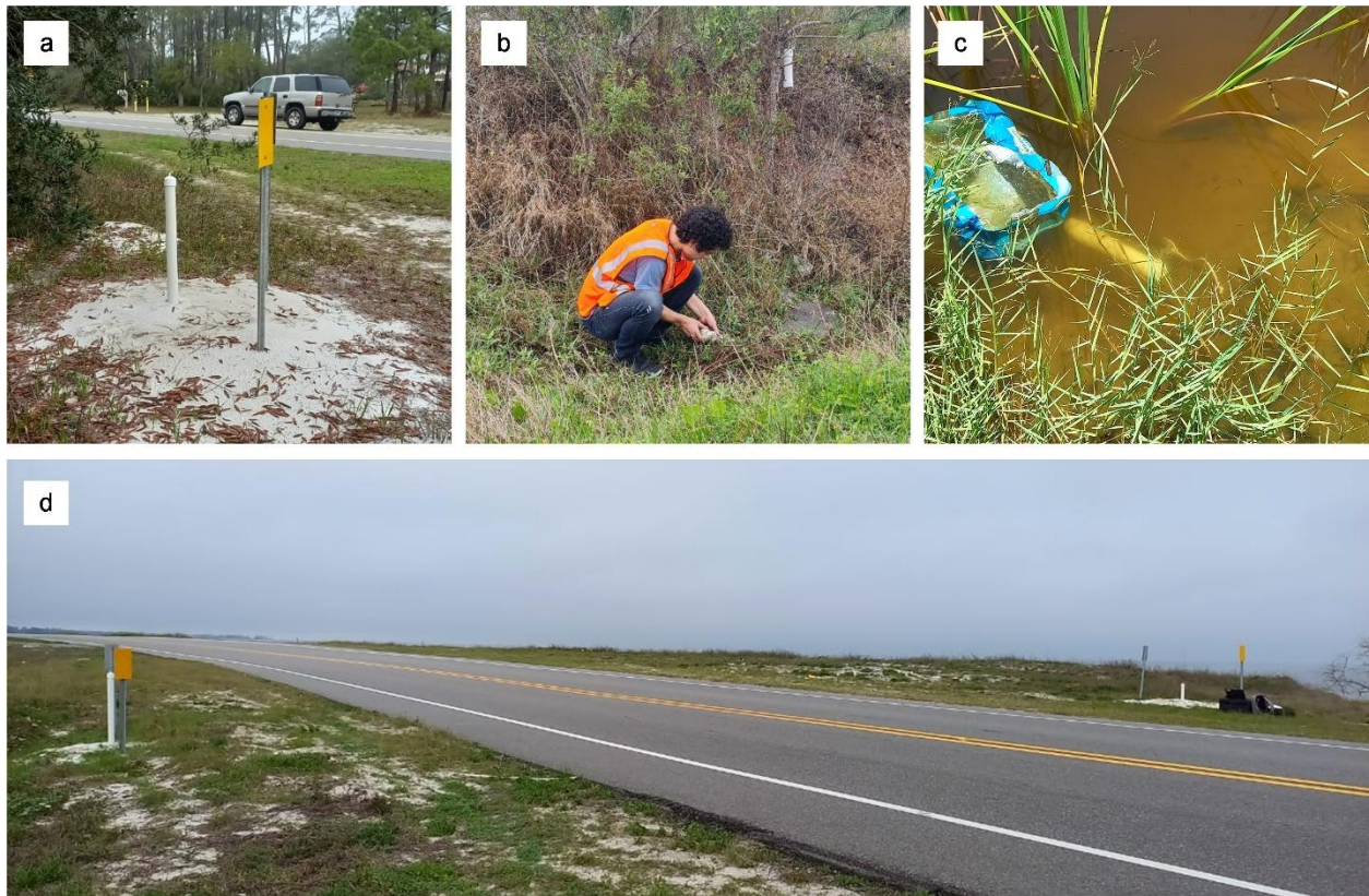
Figure 4 – a: Well set up at the Pines location, a little further away from the pavement; b: atmospheric pressure sensor hanging from a tree and a sensor/datalogger being removed from the PVC encasing in the intermittent drainage channel located at the Boat Launch location; c: Navy Cove water level downstream of a culvert; d: two wells were positioned opposite each other at the Boat Launch location.
