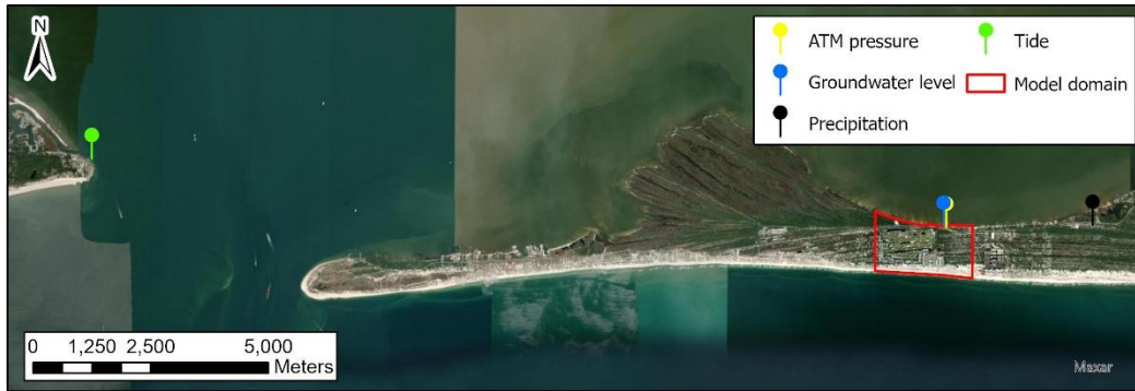
Figure 23 - Monitoring locations used in the distributed hydrologic model.
