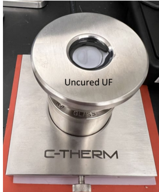
Figure 7-17 Schematic of MTPS for Uncured UF
