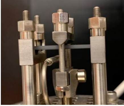
Figure 3-11 Three Points Bending Setup with Specimen
