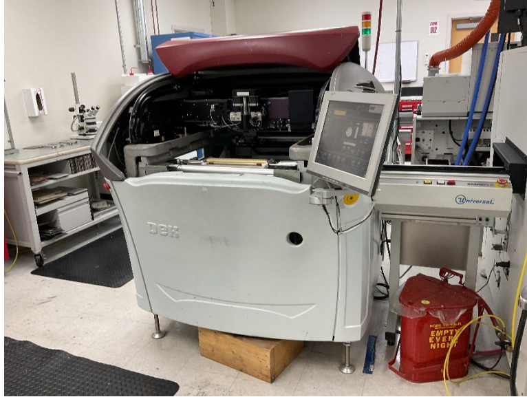
Fig. 4-5: Universal Industries' DEK Galaxy SMT stencil printer.
