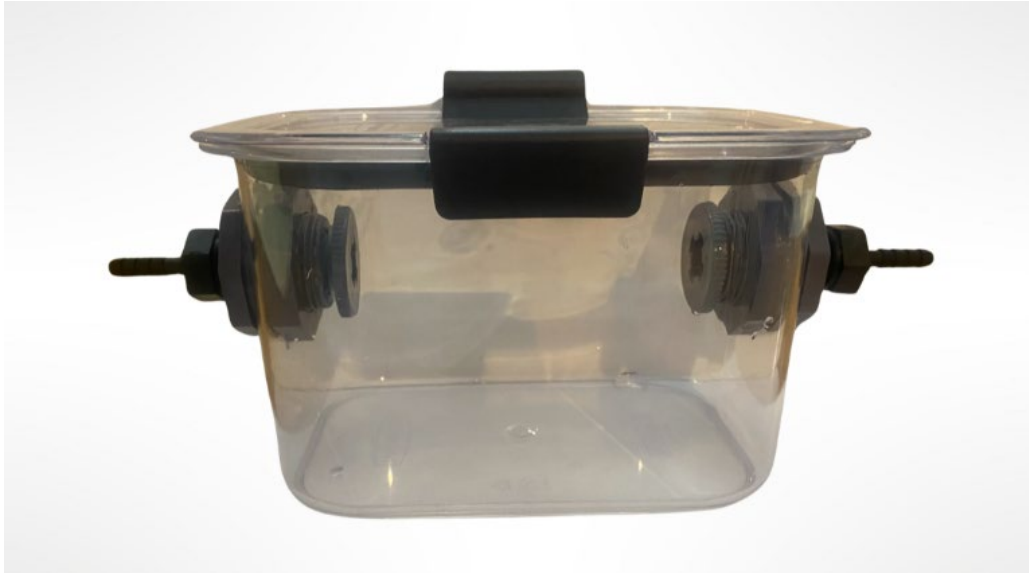
Figure 4: Control chamber where untagged beetles will be placed during trials. The chamber design allows for a 360 0 view for an accessible view of beetles when inside. The lid can be easily removed to further visualize beetles from above.
