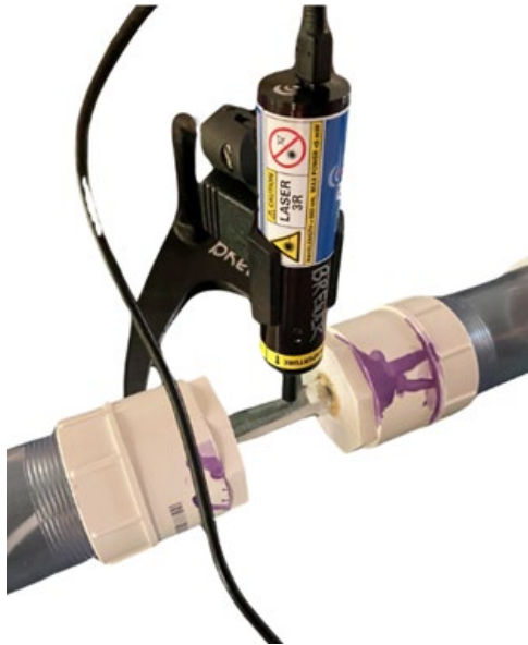
Figure 3: p-Chip scanner in between each of the control chambers which was used to continuously detect passing tagged individuals as they passed through each of the chambers.
