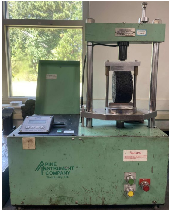
Figure 9. Tensile Strength Ratio (TSR)
