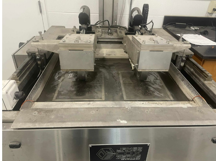
Figure 11. Hamburg Wheel Tracking Test (HWTT)
